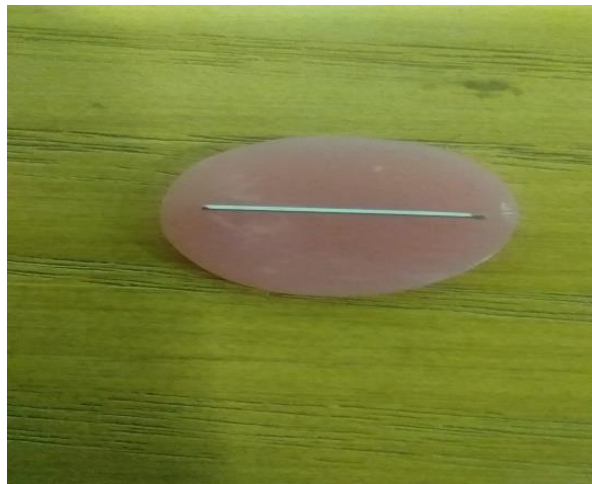
Fig 1: This is one of the samples of hardness testing of arch wire NiTi (testing by hazardous of affected and non-affected zones)
