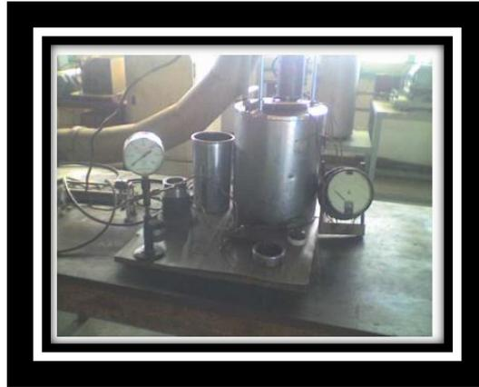
**Plate-2.2: Bomb calorimeter used for the calorific value**
