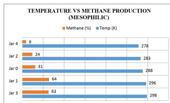
**Fig-2: Temperature VS Methane Production (Mesophilic)**
