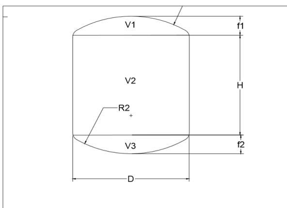
Fig-7: Geometrical Dimensions of Cylindrical Shaped Biogas Digester Body
