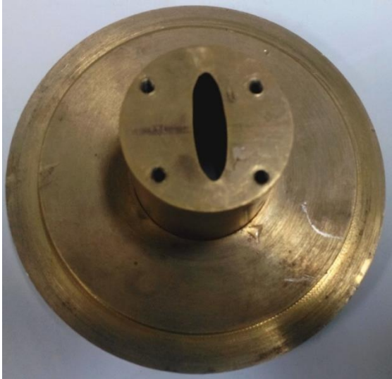
Fig-11: Mach 1.5 convergent-divergent elliptical nozzle of Aspect Ratio 3
