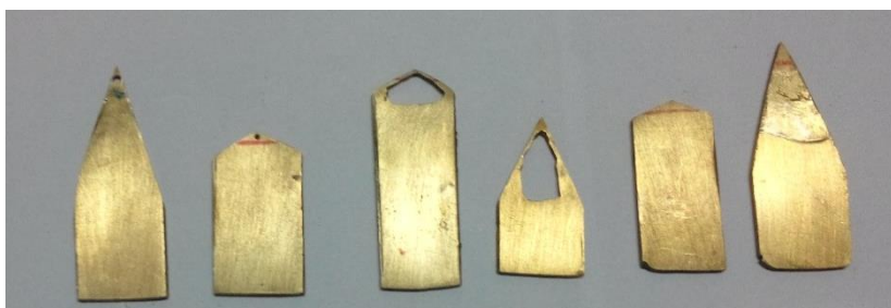
Fig-10: The tabs from left to right are Circular hole on triangular major tabs, Circular hole on triangular minor tabs, Triangular hole on triangular minor tabs, Triangular hole on triangular major tabs, Minor tabs, and Major tabs
