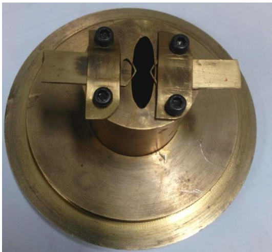
Fig-12: Nozzle configuration with triangular hole on minor tabs
