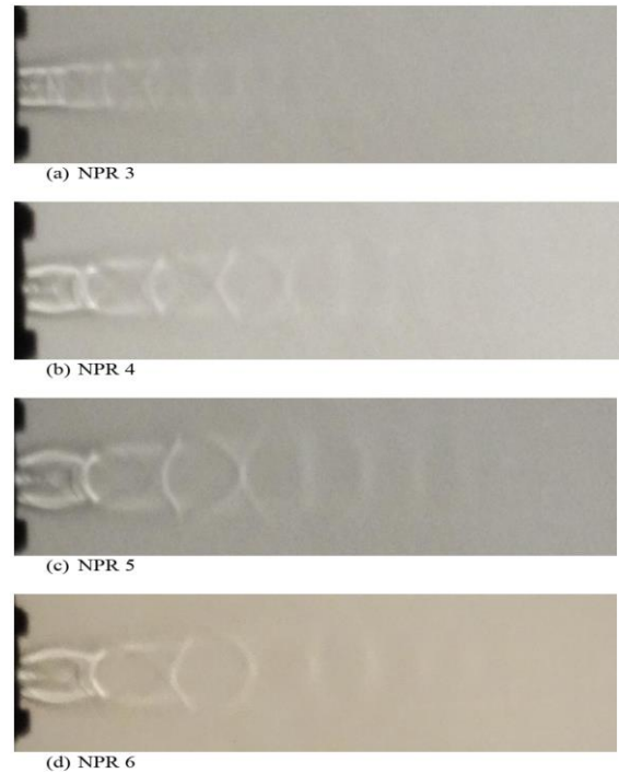
Fig-25: Shadowgraph visualization along the x-z plane for the jet controlled with triangular hole on major tabs
