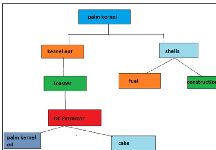
**Fig-1: Flow chart for processing of palm kernel into palm kernel oil**
