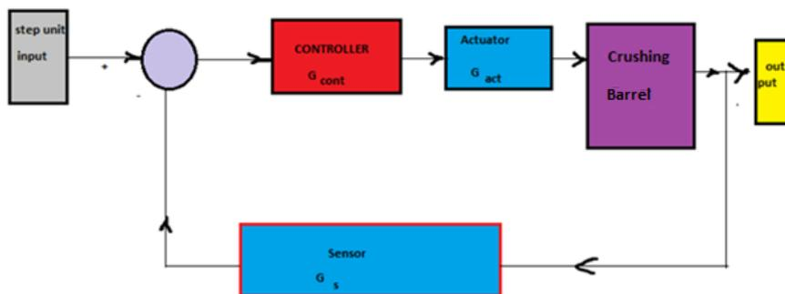
Fig-11 .Block Diagram for Crushing Barrel Model
