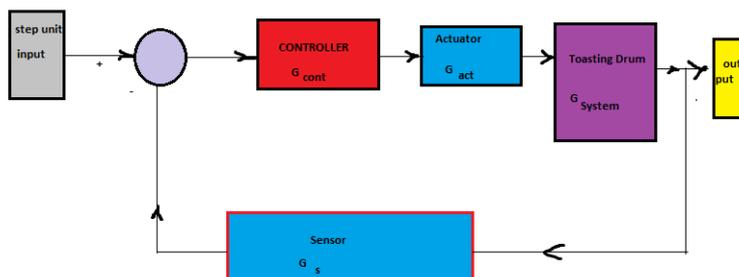
Fig-8: Block Diagramme For Toasting Drum Model
