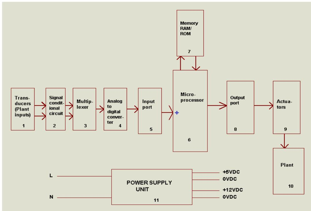
Fig-6: Detailed System Block Diagram
