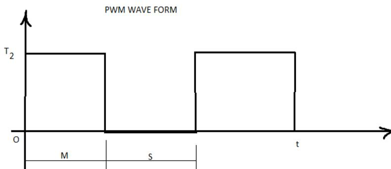
Fig-9: PWM Wave form for the blower to toasting drum.
