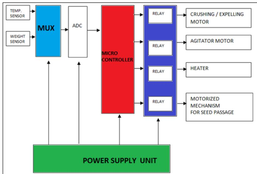
Fig-4: Block diagram of the proposed palm kernel oil Extraction System
