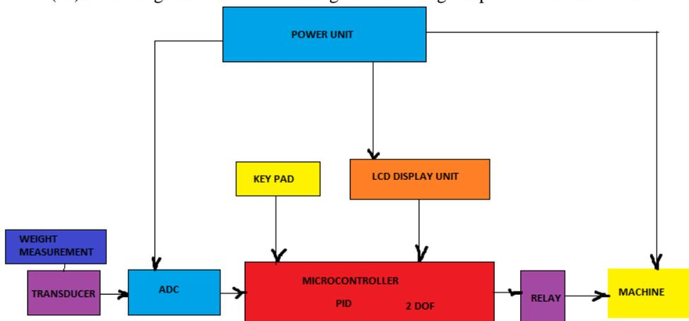
(b).Block Diagram of the Circuit Design for Weight Control into the Extractor
