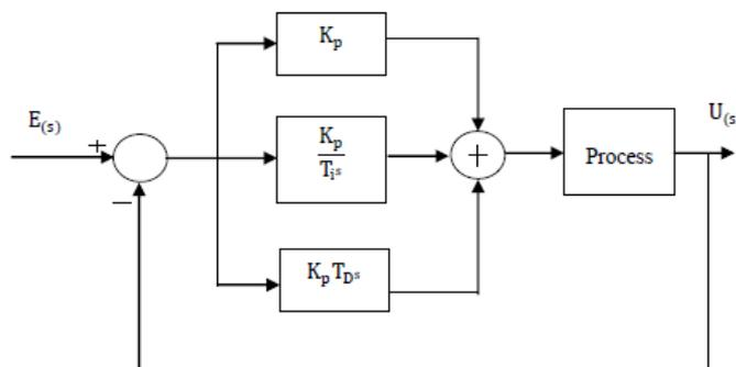
Fig-12: Block diagram of a continuous parallel PID controller
