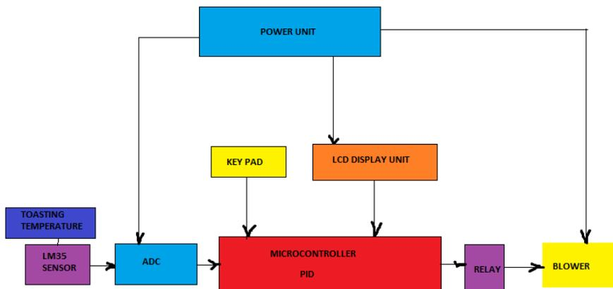
(A.)Block diagram of the circuit design for Toasting temperature chamber control.
