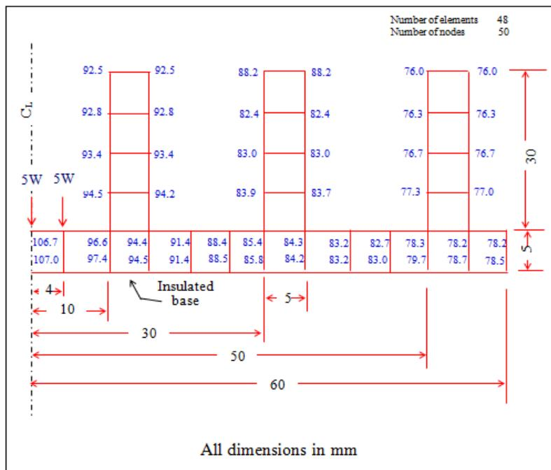
Fig-3 (b): Temperature distributions in a heat sink (case VI and V)
