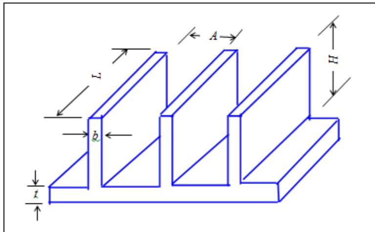
Fig-3 (a): Dimensional details of parallel fin array
