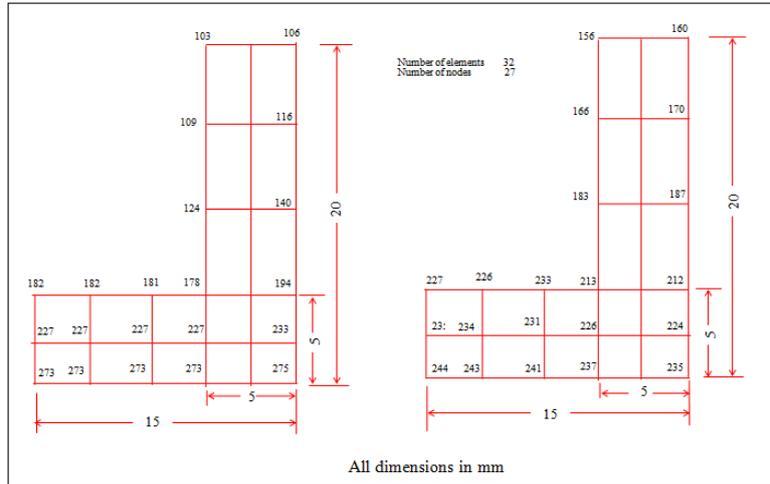
Fig-2(a): Temperature distribution in stainless steel fin (case II and III)
