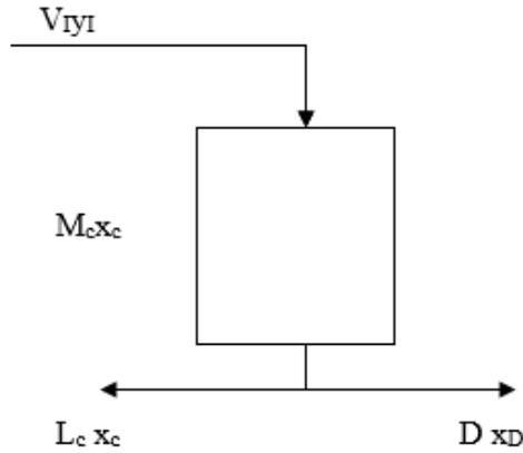
Fig-1: Material Balance around the Condenser
