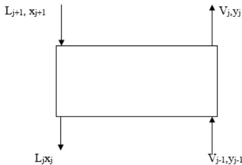
Fig-2: Material Balance around the Rectifying Sections
