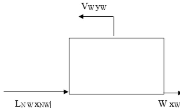
Fig-5: Material Balance around the Reboiler
