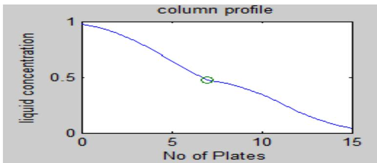
**Fig-7: MATLAB Column Profile showing Liquid composition and feed position**
