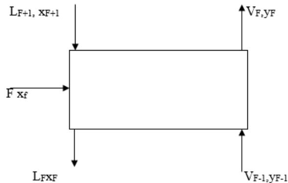
Fig-3: Material Balance around the Around Feed Plate
