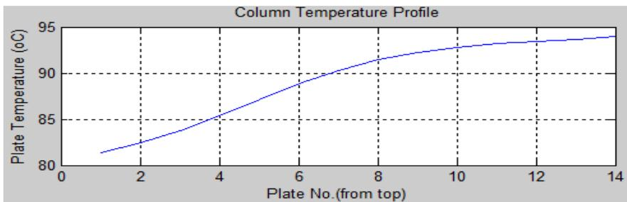
**Fig-9: Temperature Profile across the Column from Matlab**
