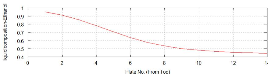
**Fig-6: Liquid Composition of the ethanol against plate from HYSYS case**
