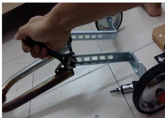
**Fig-5: Mounting the training wheels to the bicycle frame**
