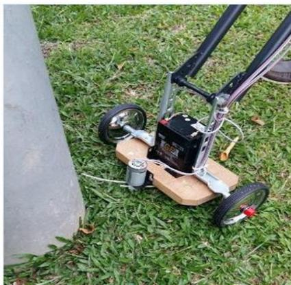
**Fig-10: Rechargeable battery attached to the base**
