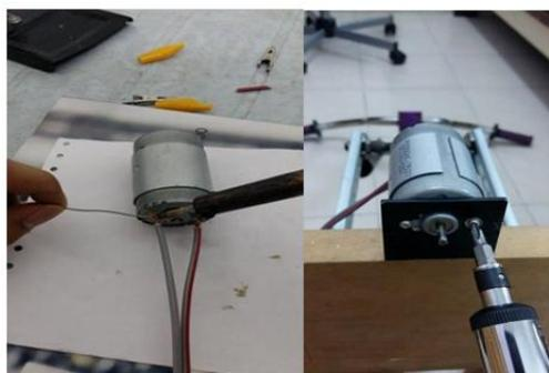
**Fig-8: Attaching the soldered electric motor to the base**
