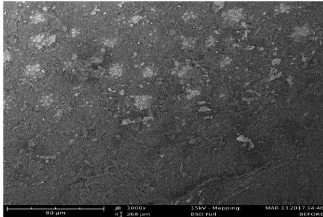
Fig-2: SEM analysis of fresh palm kernel shell before scrubbing process
