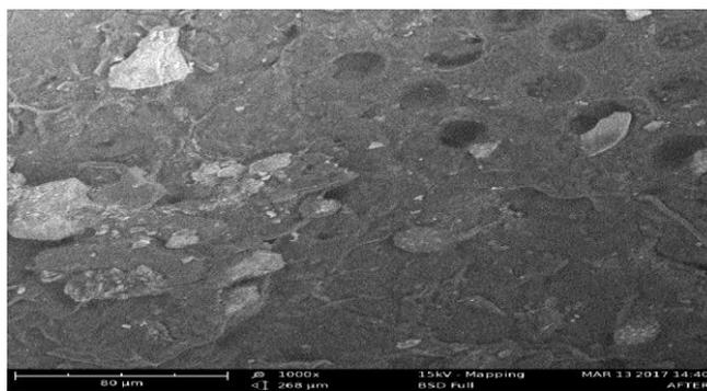
Fig-3: SEM diagram showing increased macro pores after scrubbing process.
