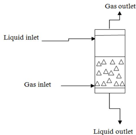
Fig-4: schematic diagram of biogas scrubber
