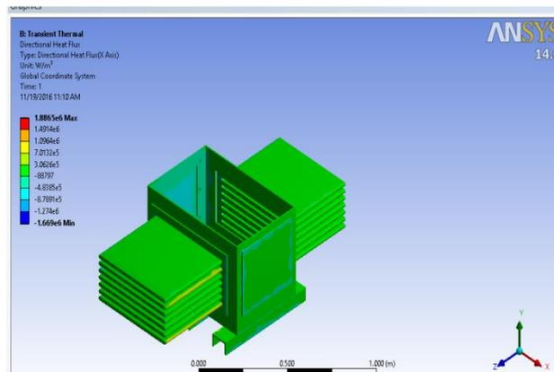
Fig-21: Direction a heat flux distribution
