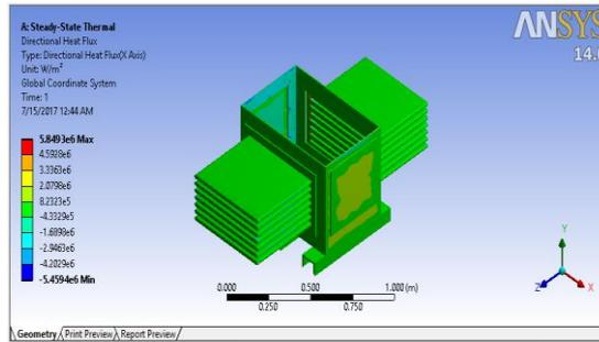
Fig-10: Directional heat distribution
