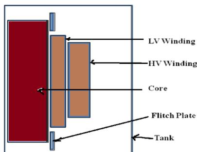
**Fig-2: dimensional transformer cross section showing essential parts**
