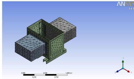
Fig-14: 3-D Mesh Form of the Cascade Model
