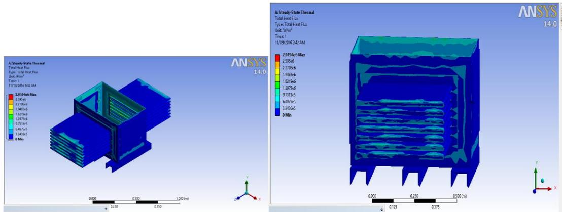
Fig-17: Total heat flux distribution
