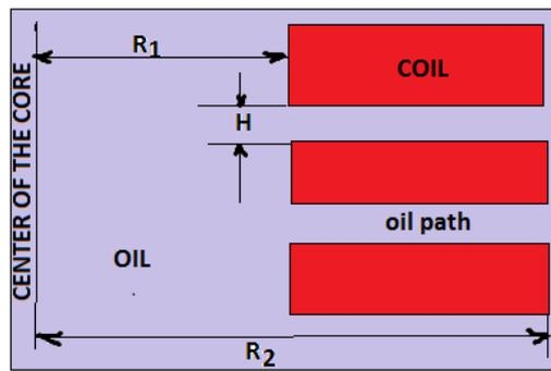
Fig-4: A Schematic Diagram of Disc Windings in Oil Data Calculation
