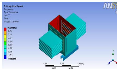
Fig-8: Temperature Distribution
