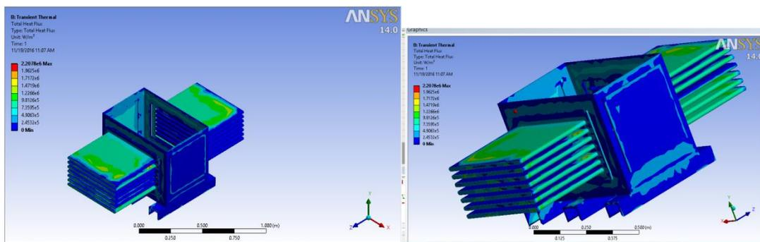
Fig-20: Total heat flux distribution in the cascade showing heat desipation
