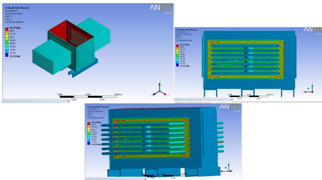
Fig-16: Temperature distribution in the model
