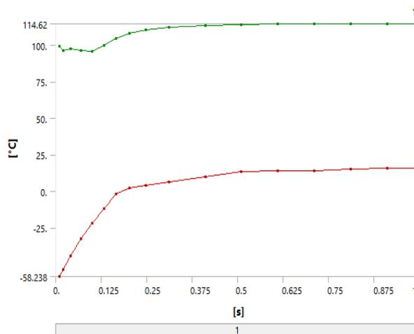
Fig-26: Minimum and maximum temperature distribution in the cascade
