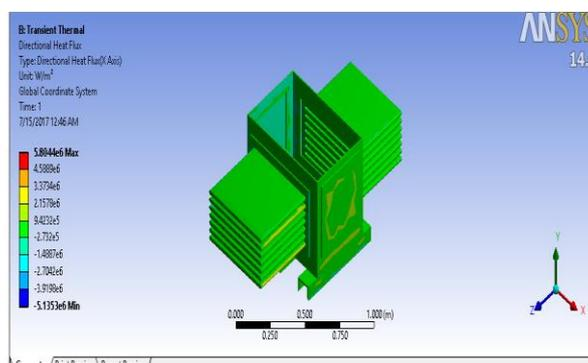
Fig-13: Directional heat flux
