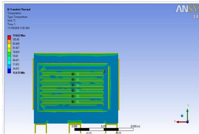
Fig-19: 3-D view of Temperature distribution in the cascade
