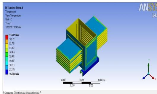
Fig-11: Temperature distribution
