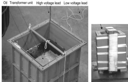
Fig-3: pictorial view of an oil filled cascaded transformer
