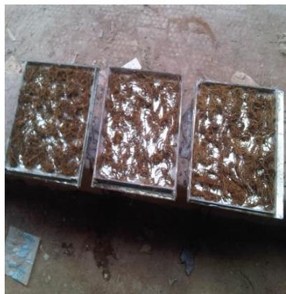
**Fig-8: Composite being prepared from jute fiber reinforced with polyester.**
