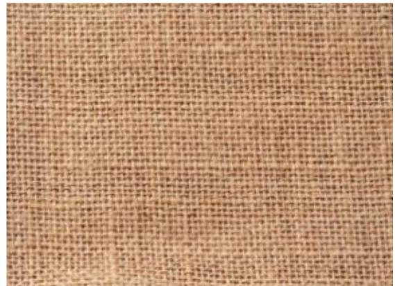
**Fig-5: Alkaline treated Jute Fiber**
