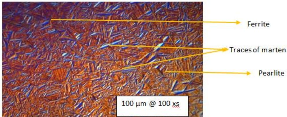
Fig-13d: Sample of D= 45mm, H= 40mm @ surface temperature 458<sup>0</sup>C
