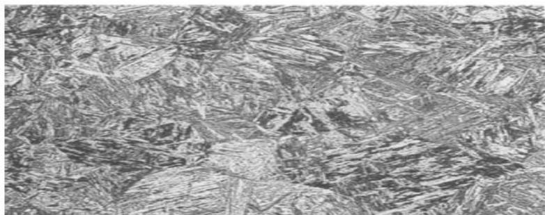
Fig-7: Microstructure of a typical martensite at 200x [6]
