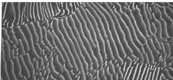
Fig- 5: Micrograph of pearlite showing ferrite and cementite 10,000x [5]
