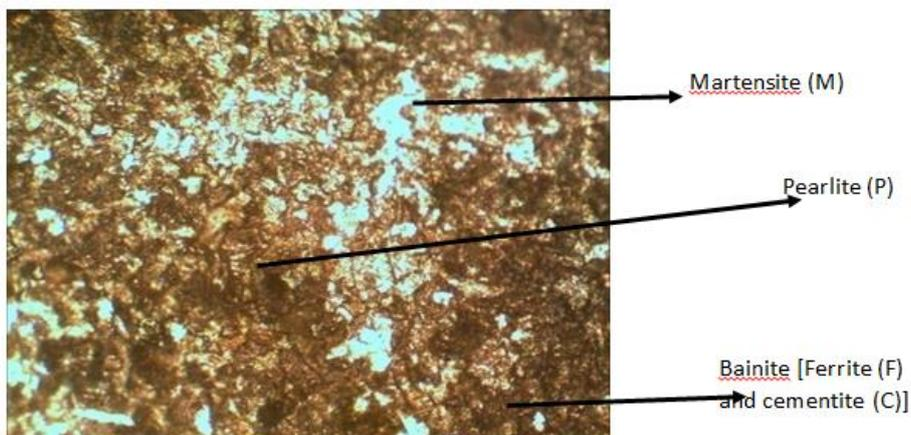
**Fig-10: Microstructure of workpiece before heating and impingement, 100 x magnifications**
