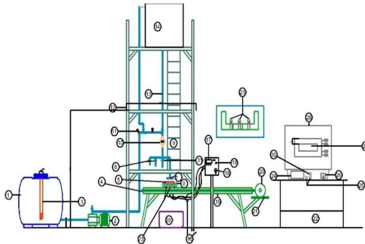
**Fig-8: Schematic diagram of pilot plant for this research in MMEFL**
