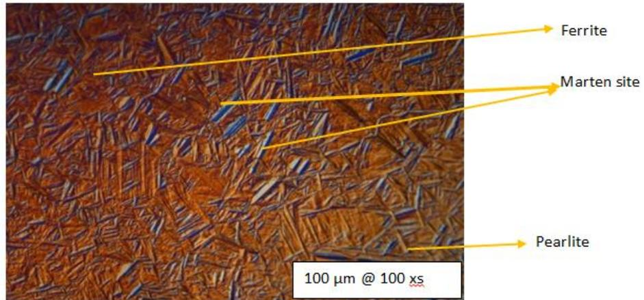
**Fig-12d: Sample of D= 45mm, H= 70mm @ surface temperature 438<sup>0</sup>C**
