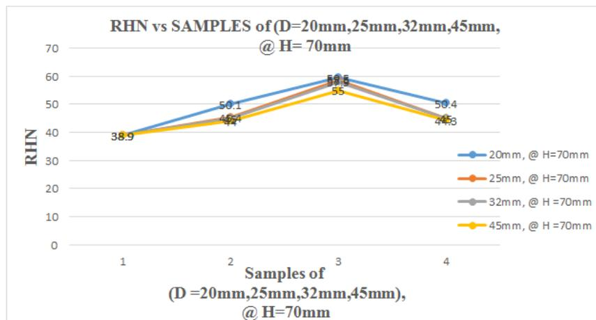
Fig-14b: Graphs of Comparative of D= 20mm, 25mm, 32mm and 45mm at impingement gap H =70mm
