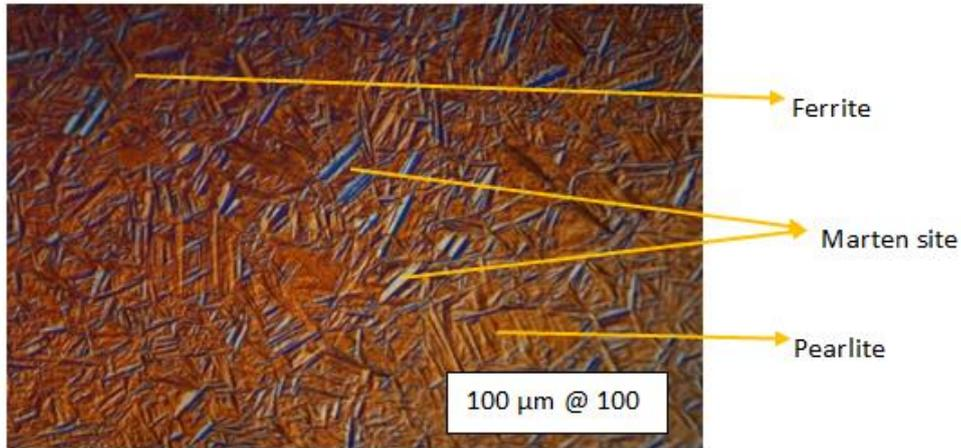
Fig-13c: Sample of D= 32mm, H= 40mm @ surface temperature 470<sup>0</sup>C
