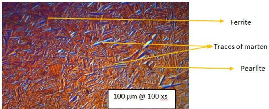
**Fig-12c: Sample of D= 32mm, H= 70mm @ surface temperature 440<sup>0</sup>C**
