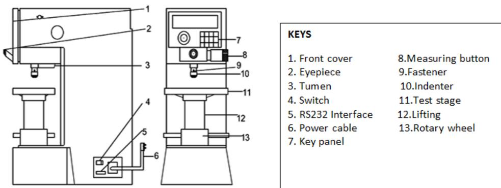
**Fig-11: Rockwell Hardne Test Machine**
