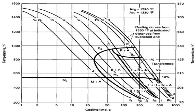
Fig-6: The CCT Diagram for type 4340 Steel Austenitized at 845<sup>0</sup>C [3]
