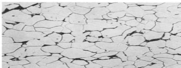
Fig-4: Micrograph of pearlite in low carbon steel 1000x [5]
