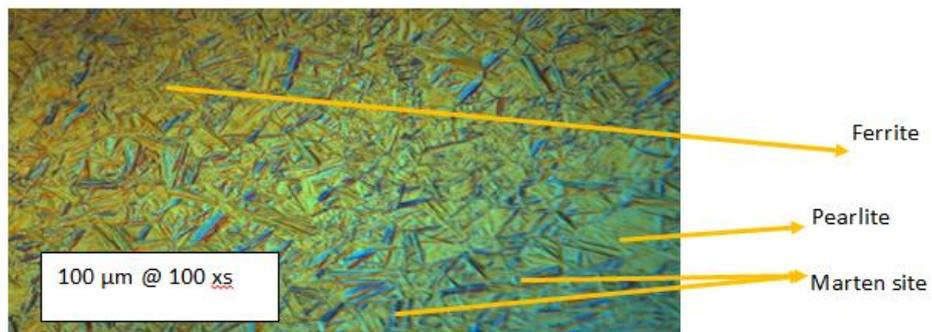
**Fig-12b: Sample of D= 25mm, H= 70mm @ surface temperature 463<sup>0</sup>C**
