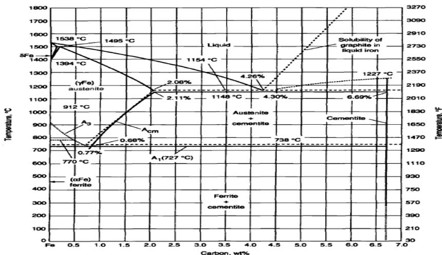
Fig-3: Iron carbon binary phase diagram [4]
