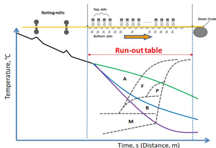
**Fig-1:** Schematic of hot rolling mill of steel plates and strips. The schematic plot shows temperature variation versus time and its effect on the phase transformation of austenite decomposition. A: austenite, F: ferrite, P: pearlite, B: bainite, M: martensite.
