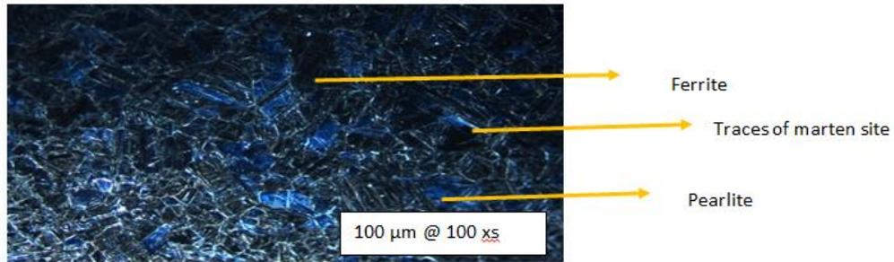
**Fig-12a: Sample of D= 20mm, H= 70mm @ surface temperature 469<sup>0</sup>C**
