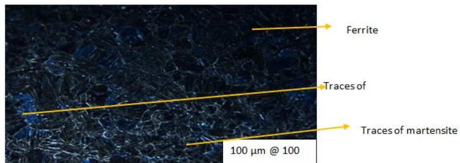
**Fig-13a: Sample of D= 20mm and H= 40mm @ surface temperature 500<sup>0</sup>C**
