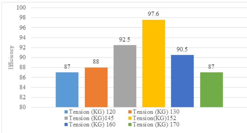
Fig-5: Warp Tension Vs Efficiency
