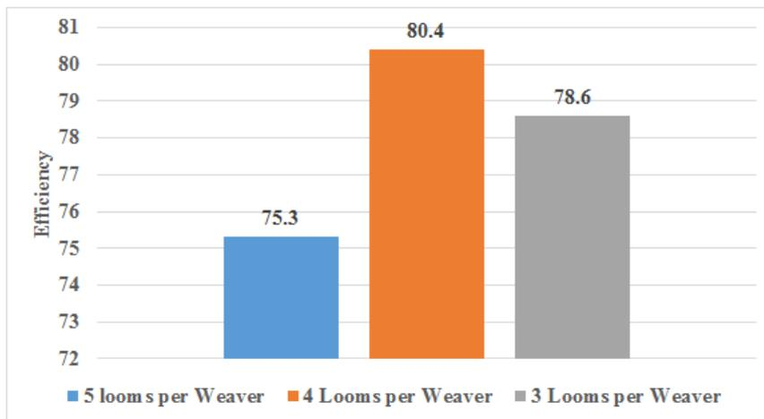
**Fig-13: Analysis of Efficiency by Loom Allocation**
