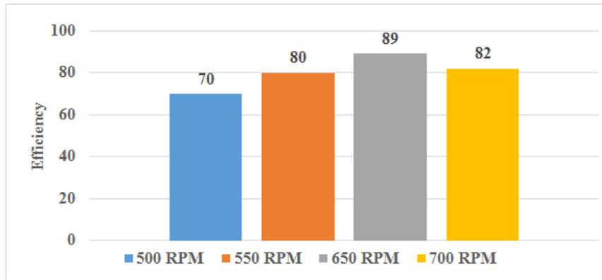
**Fig-17: Analysis of Efficiency by Speed**
