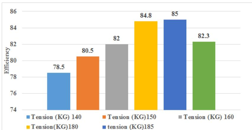
Fig-6: Warp Tension Vs Efficiency
