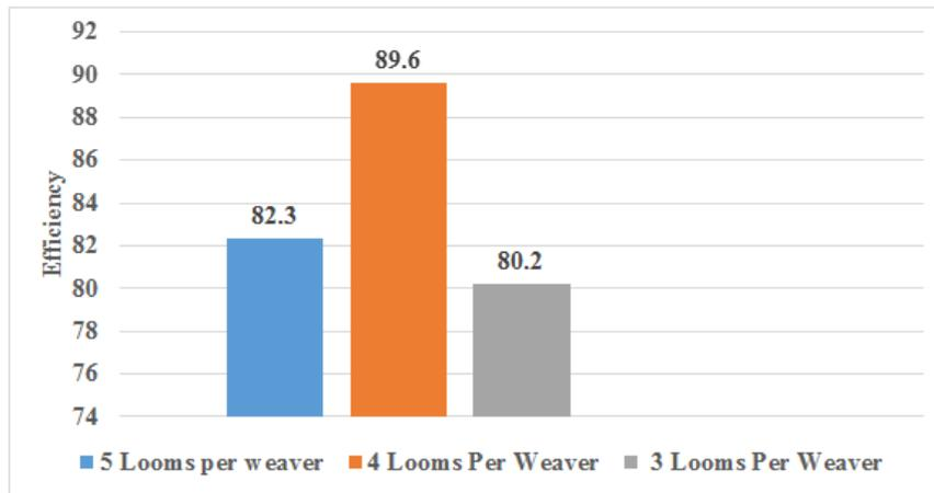
**Fig-12: Analysis of Efficiency by Loom Allocation**
