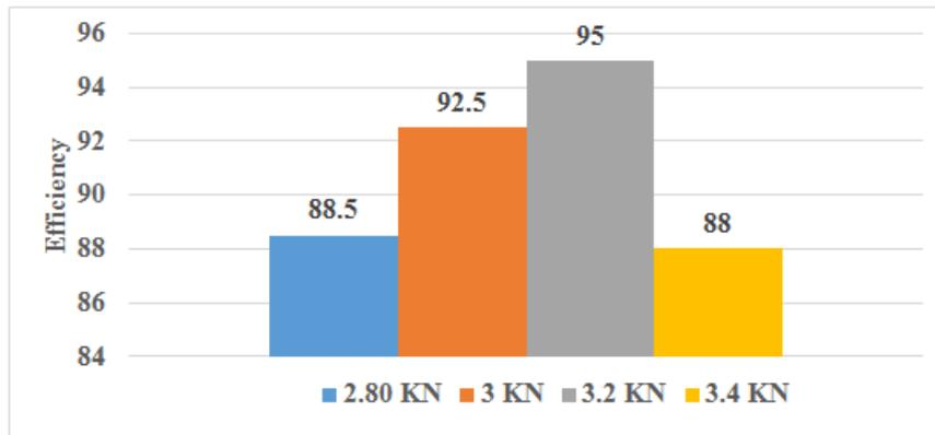
**Fig-21: Warp Tension Vs Efficiency**
