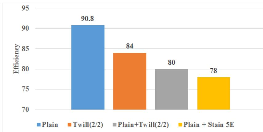
Fig-8: Weave Type Vs Efficiency
