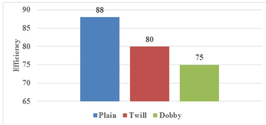
Fig-22: Weave Type Vs Efficiency
