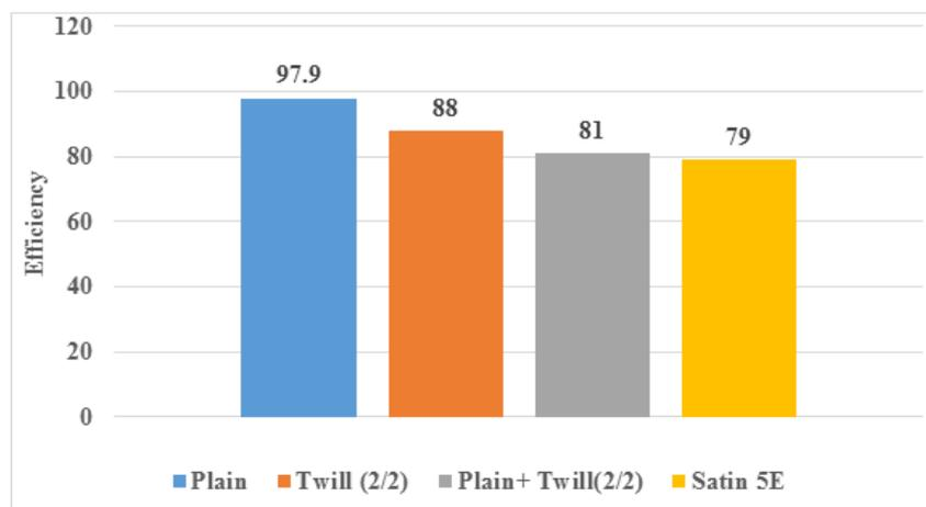
Fig-7: Weave Type Vs Efficiency
