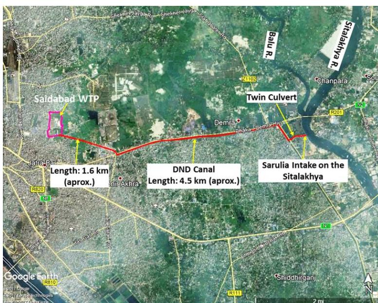
**Fig-1: Raw water source and its transmission network from Sitalakhya river through DND canal to plant**
