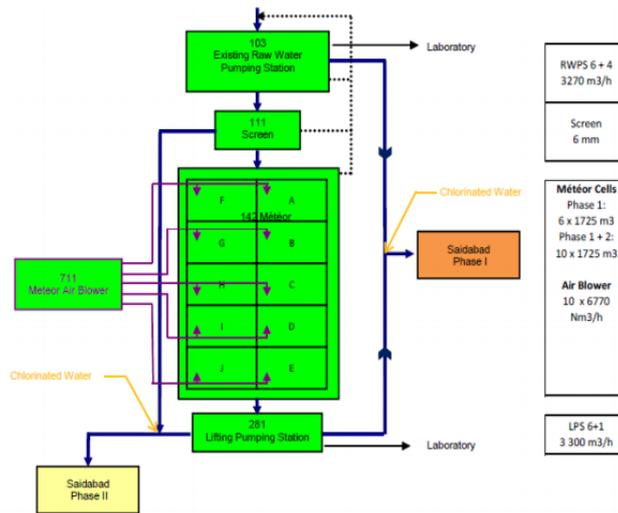
Fig- 2: Meteor Reactors
