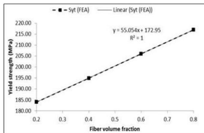
**Fig-4: Variation of tensile strength with fiber fraction volume**
