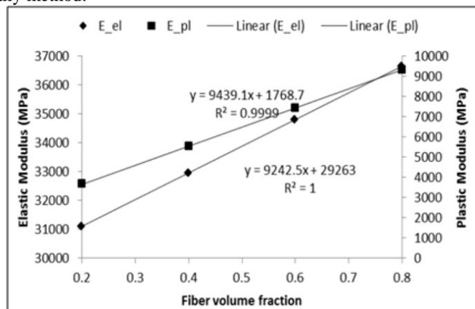
Fig-5: Variation of elastic and plastic moduli with fiber volume fraction
