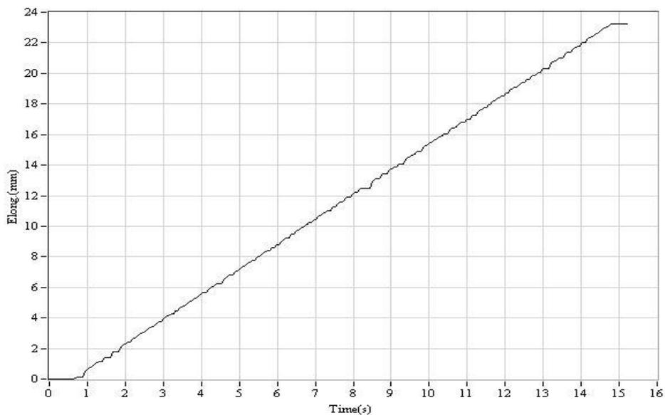
Fig-14: Elongation Vs Time Plot at Optimum strength of 10% concentration at 50°C
