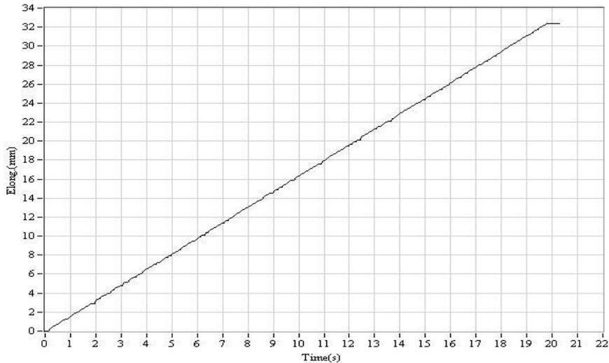
**Fig-10: Elongation Vs Time Plot at Optimum Strength of 2% concentration**
