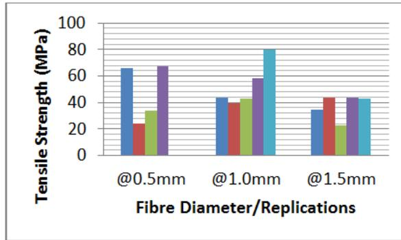
Fig-4: Strengths at drying temperature of 50<sup>0</sup>C at varying diameter of fibres
