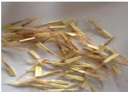
**Fig-2: Samples after Tensile Testing Process**
