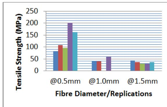
Fig-5: Strengths at drying temperature of 80<sup>0</sup>C at varying diameter of fibres
