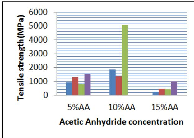
Fig-12: Strengths at varying Acetic Anhydride concentrations at acetylation temperature 50°C
