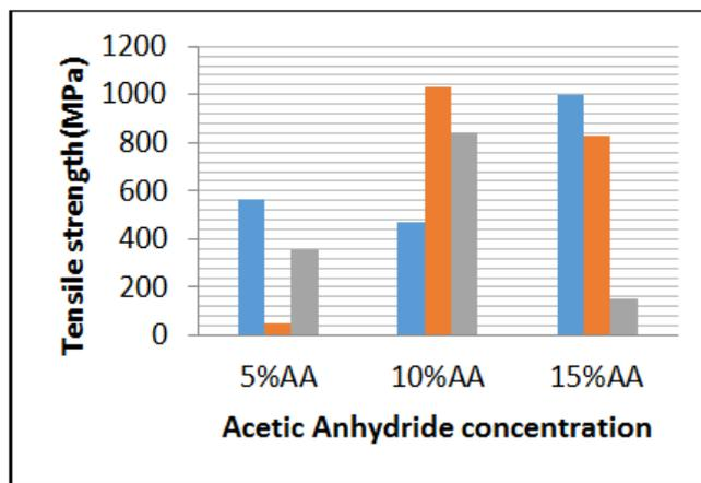
Fig-13: Strengths at varying Acetic Anhydride concentration at acetylation temperature 30°C
