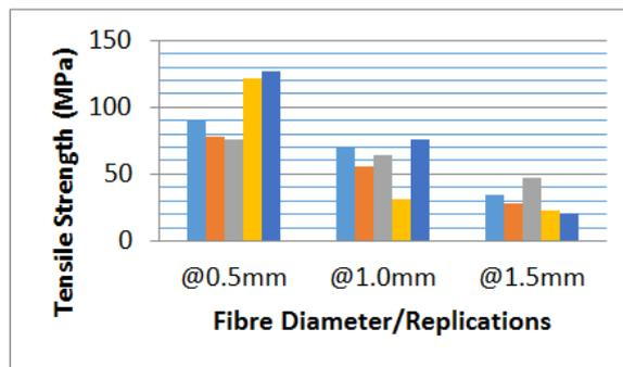
Fig-6: Strengths at drying temperature of 100<sup>0</sup>C at varying diameter of fibres
