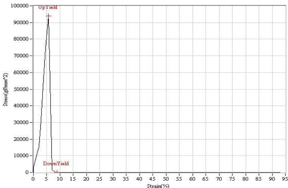
**Fig-15: Stress Vs Strain Plot at Optimum Strength of 10% Concentration at 50°C**
