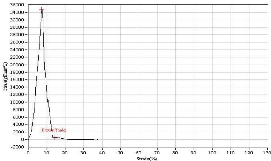
**Fig-11: Stress Vs Strain Plot at Optimum Strength of 2% Concentration**
