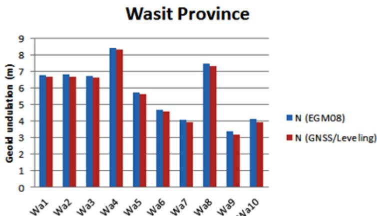
**Fig-3: Chart Show the Difference between Geoid Undulation (EGM08) and Geoid Undulation from (GPS/Leveling)**
