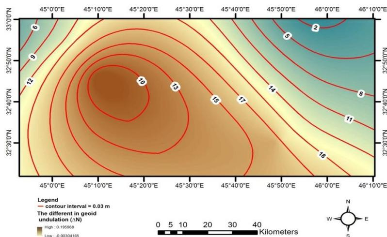
**Fig-4: Contour Map Show the Different in Geoid Undulation**
