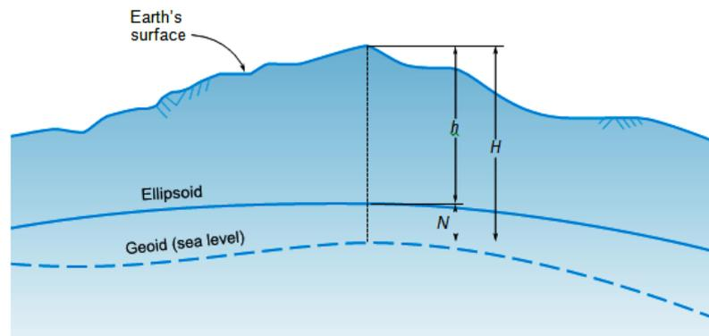
**Fig-2: the Relationship between geoid, ellipsoid and orthometric Height**
