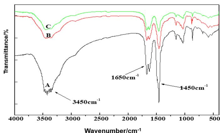
Fig-5: The FTIR spectrogram of composite membranes under different matrix conditions (A: CMC-1; B: CMC-2; C: CMC-3)
