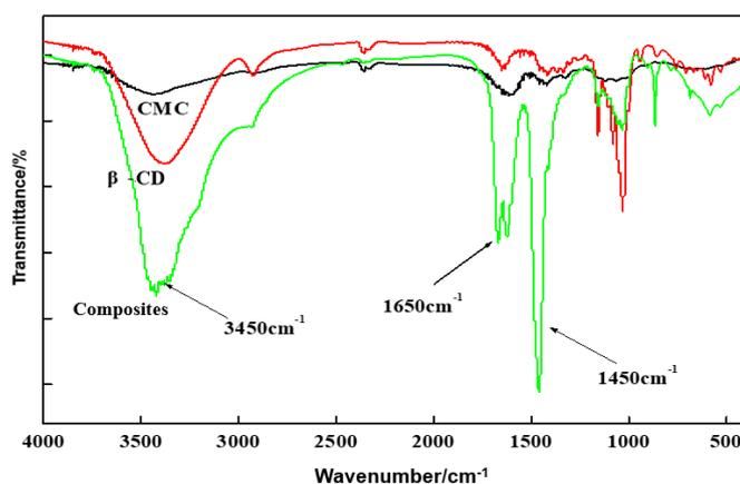
Fig-4: The FTIR spectrogram of CMC,  $\beta$ -CD, and  $\beta$ -CD/CMC membrane composites
