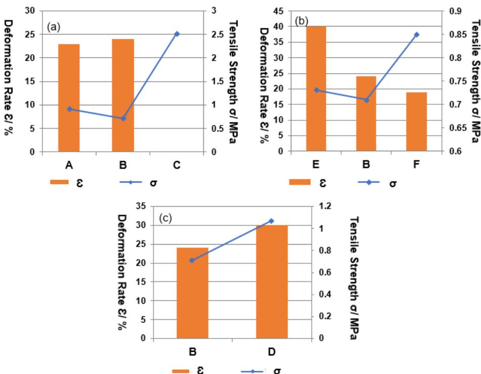
Fig-3: The mechanical properties of composites with 0.5g  $\beta$ -CD added under different matrix conditions (a: the mixing time; b: the content of  $\text{SiO}_2$ ; c: frozen or not)
