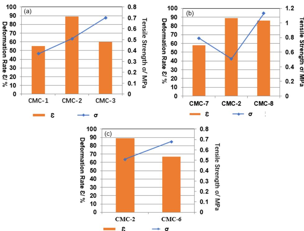
**Fig-1: The mechanical properties of composites under different matrix conditions (a: the mixing time; b: the content of  $\text{SiO}_2$ ; c: frozen or not)**
