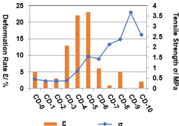
Fig-2: The mechanical properties of composites under different  $\beta$ -CD content
