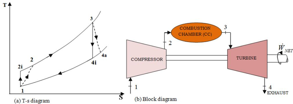
**Fig-2: Temperature- entropy (T-s) and block diagrams of a real GT engine cycle**
