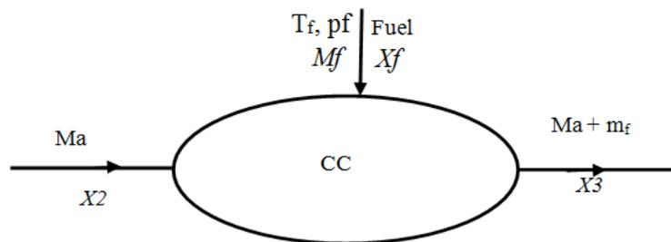
**Fig-4: Exergy balance in the combustion chamber**
