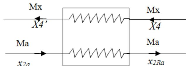
**Fig-5: Exergy balance in the regenerator**
