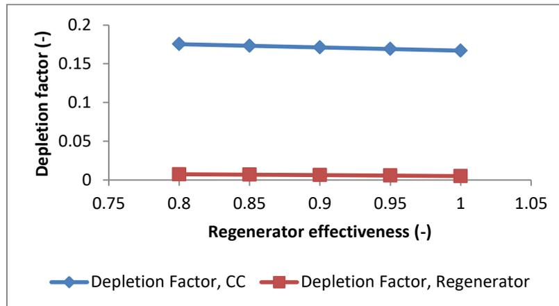
Fig-7: Depletion factor for regenerative cycle components at different values of regenerative effectiveness
