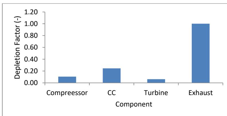
**Fig-6: Depletion factors of simple cycle gas turbine components**
