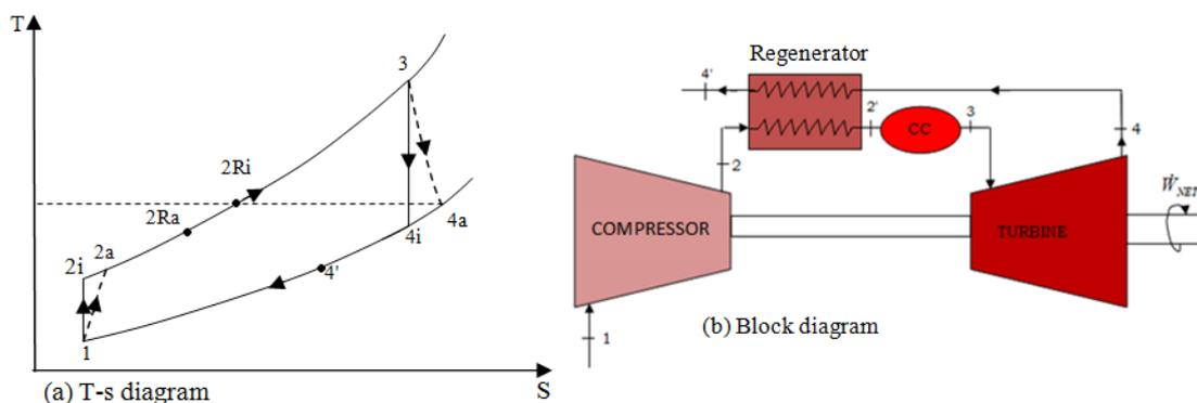
**Fig-3: T-s and block diagrams of a regenerative gas turbine engine cycle**
