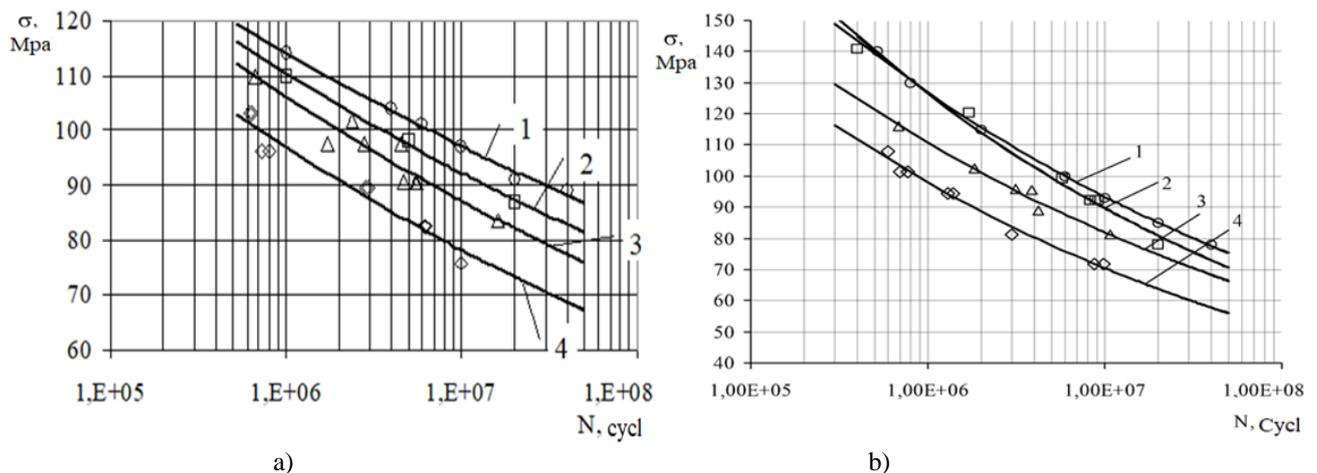
**Fig-4: Fatigue curves at different temperatures and at various frequencies (testing frequency – 9 kHz) for a) Al4 alloy and b) Al7 alloy (1- 20°C; 2- 155°C; 3- 270°C; 4- 340°C)**
