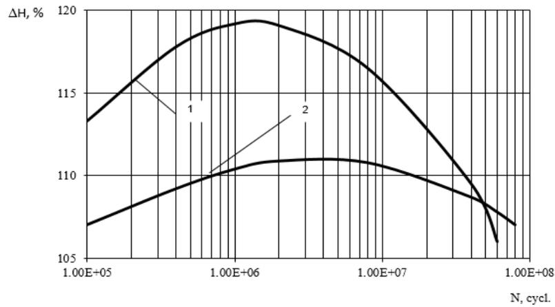
**Fig-9: Influence of the magnitude of alternating bending on the kinetics of microhardness of the Al4 alloy (0.3 kHz). 1) 87.5 MPa; 2) 62.5 MPa**
