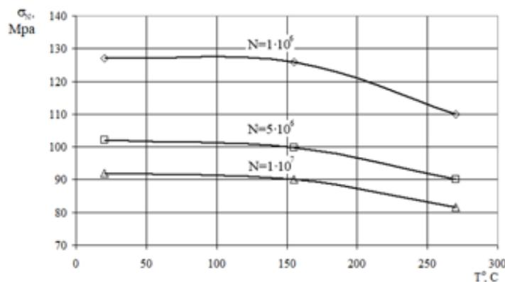
**Fig-5: Influence of the test temperature on the behavior of endurance limits for the Al7 alloy**
