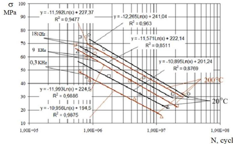
**Fig-6: Influence of Loading frequency and temperature on fatigue characteristics of AK8M3 alloy (cast state)**
