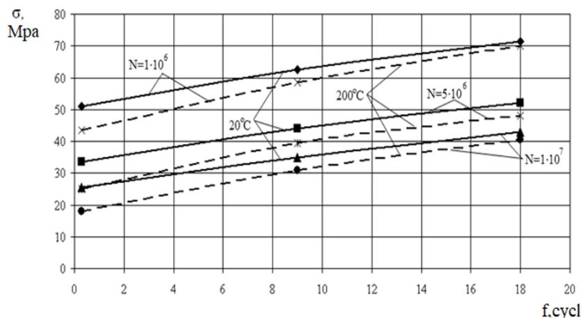
**Fig-7: Endurance limits of the AK8M3 limits at various frequencies and with various loading bases**
