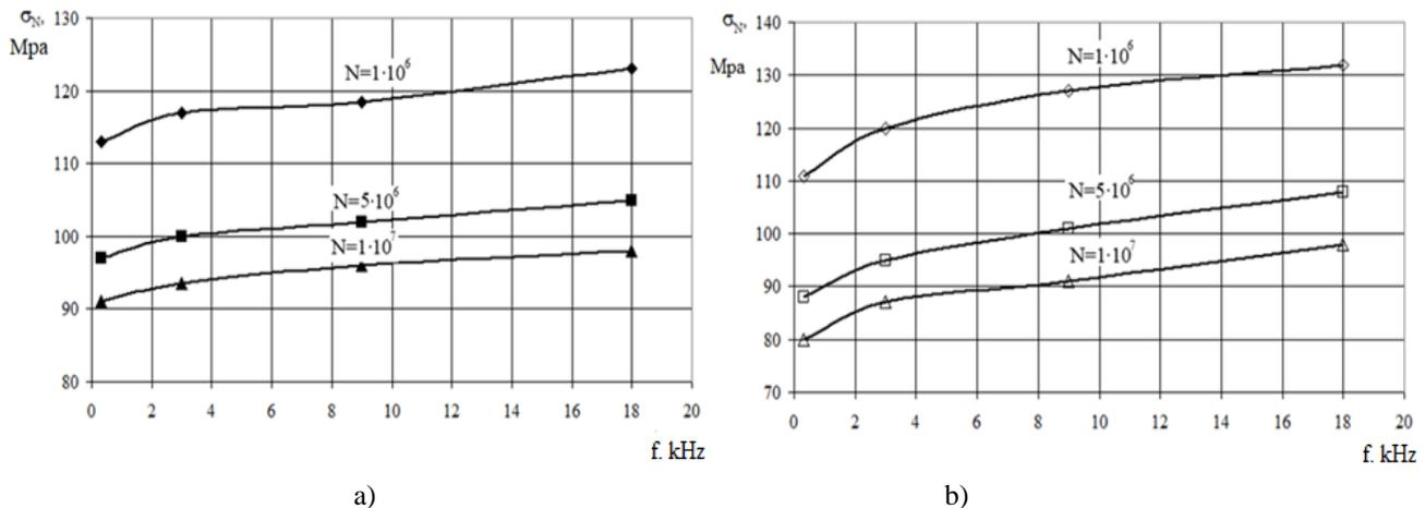
**Fig-2: Endurance limits at various loading frequencies for a) Al4 alloy b) Al7 alloy**
