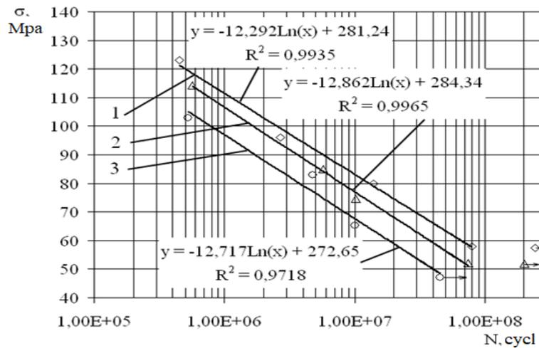
**Fig-3: Fatigue curves of the AK9M2 alloy (testing frequency 18 kHz)**
