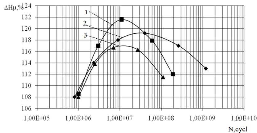
**Fig-11: Influence of temperature on the microhardness kinetics of AK9M2 alloy. 1) 20°C; 2) 100°C; 3) 250°C**
