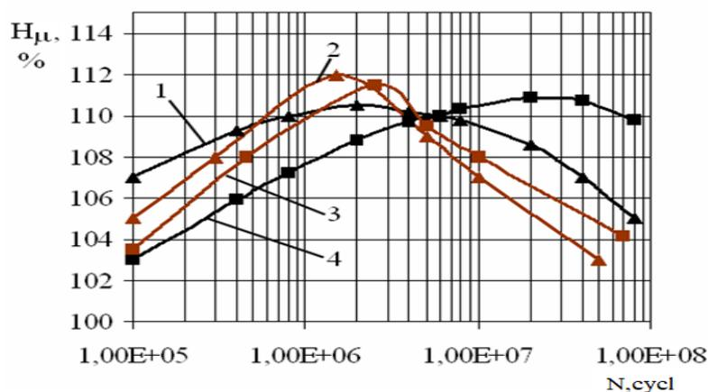
**Fig-12: Change in microhardness of the AK9M2 alloy at various test temperatures and frequencies. 1) 0.3 kHz (20°C); 2) 0.3 kHz (200°C); 3) 18.0 kHz (200°C); 4) 18.0 kHz (20°C)**
