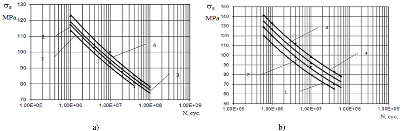
**Fig-1: Fatigue curves under alternating bending at 1) 0.3 kHz; 2) 3.0 kHz; 3) 9.0 kHz; 4) 18.0 kHz for a) Al4 and b) Al7 alloy**
