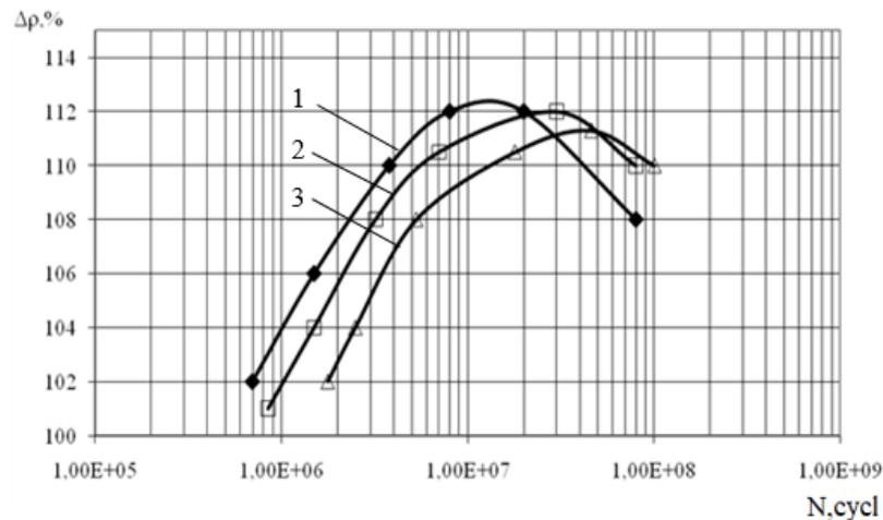
**Fig-10: Influence of the frequency of alternating bending on the kinetics of density of dislocations of the AK9M2 alloy. 1) 0.3 kHz, 2) 9 kHz, 3) 18 kHz**
