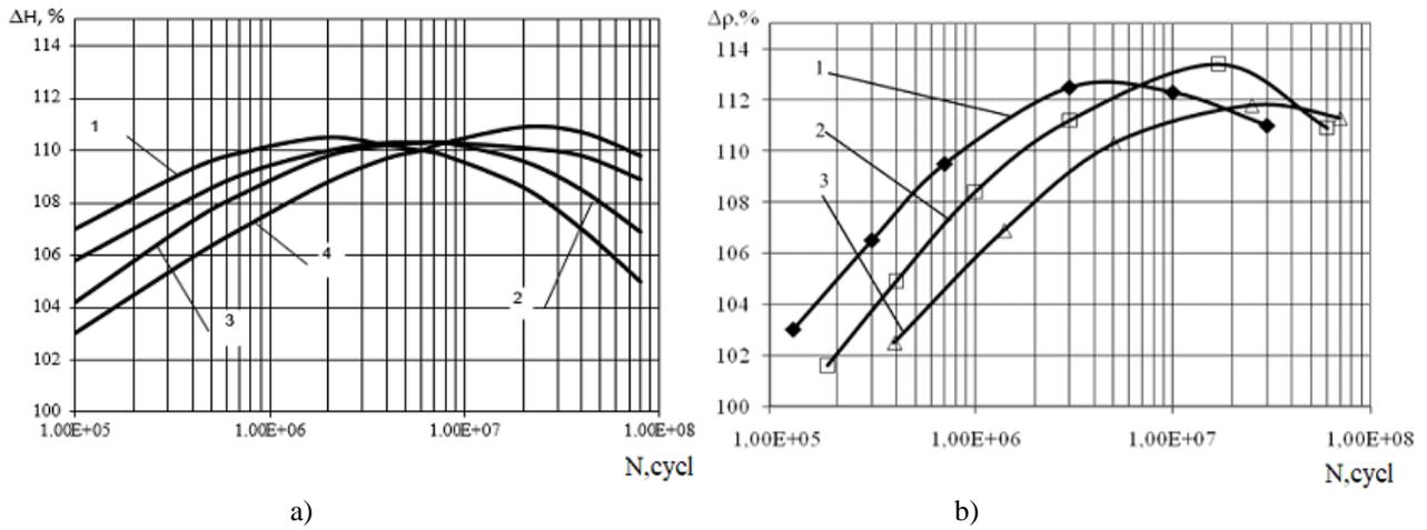
**Fig-8: Influence of the frequency of alternating bending on the kinetics on the Al4 alloy for: a) microhardness 1) 0.3 kHz, 2) 3.0 kHz, 3) 9 kHz, 4) 18 kHz and b) dislocation density 1) 0.3 kHz, 2) 9 kHz, 3) 18 kHz**
