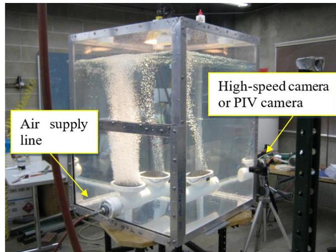
**Fig-1: Air diffuser experimental setup**
