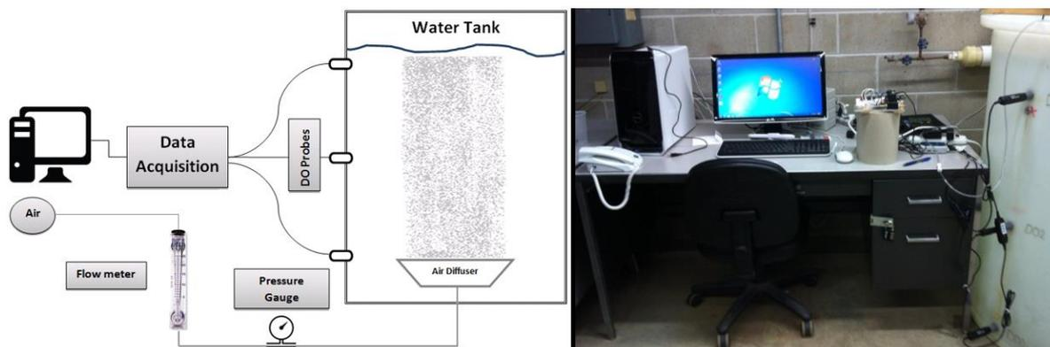
**Fig-2: Dissolved Oxygen Experimental Setup Layout**
