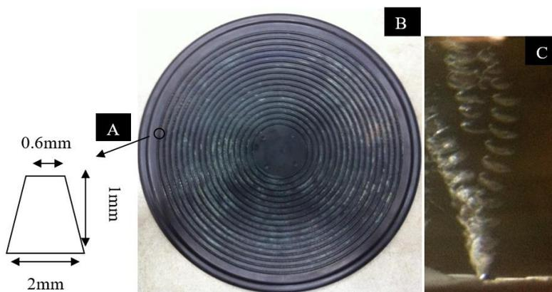
**Fig-3 (a): Nozzle design and dimension; (b) sharp nub membrane; (c) bubbles splitting due to nozzle effect**
