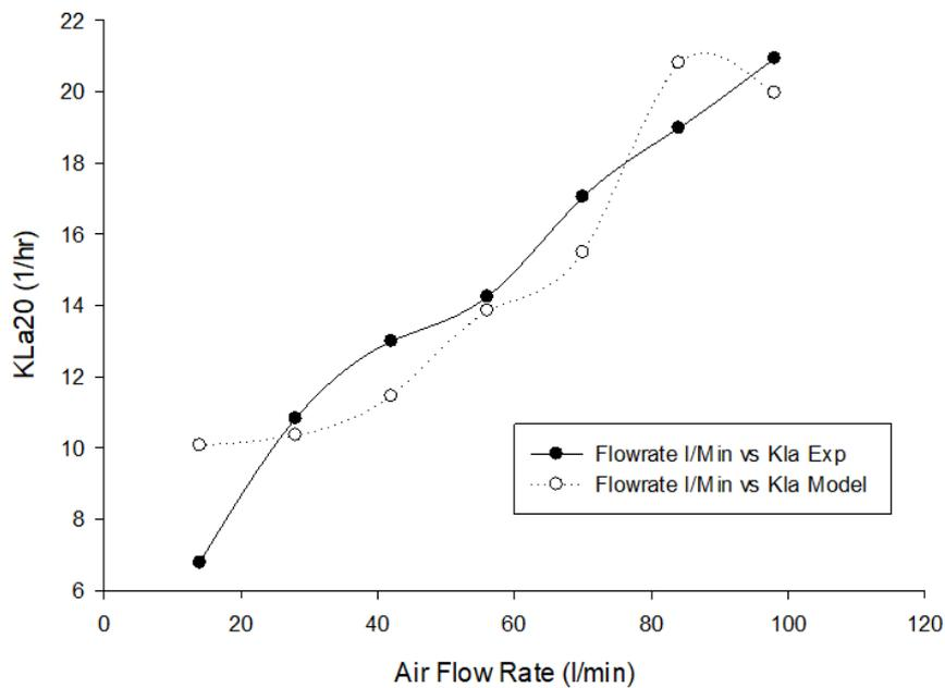
**Fig-4:  $K_{La20}$  versus airflow rate**
