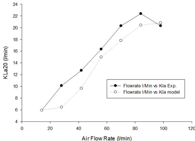
**Fig-5: Sharp Nub membrane  $K_L a_{20}$  values using the proposed model and experimental results**
