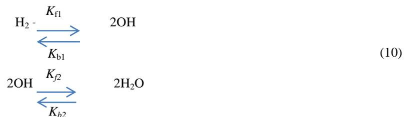
It is important to say that nitrogen is present in the calculation but is assumed inert. So four species are  $\text{H}_2$ ,  $\text{O}_2$ ,  $\text{H}_2\text{O}$ ,  $\text{N}_2$ . The  $K_f$  values are forward reaction rates and  $K_b$  values are reverse reaction rates. The reverse rates can be found, given the forward and the equilibrium constant  $K$  for each reaction as
