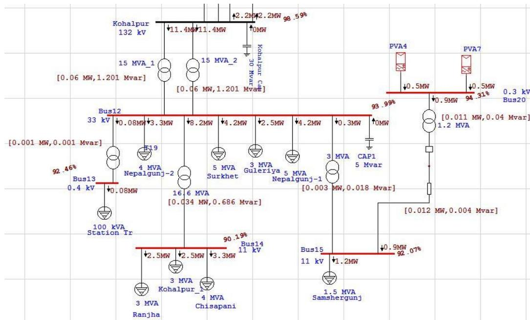
Fig-4: Load flow analysis of the grid after synchronization of solar PV
