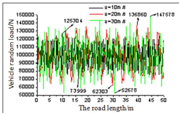
**Fig-4: The random load curve of truck**
