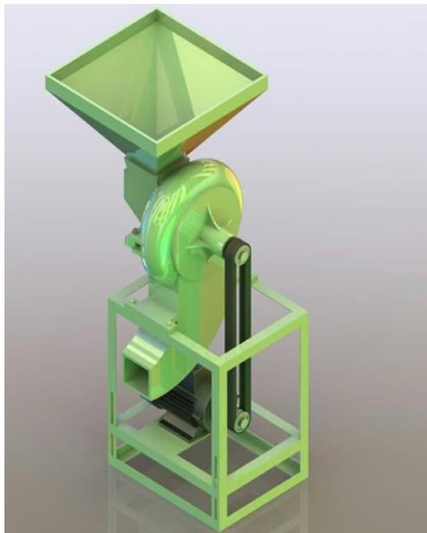
**Fig-2: Isometric Model View of Cereal Crushing Machine**
