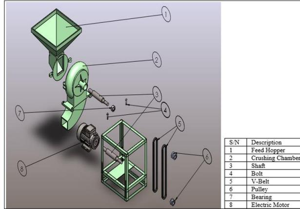
**Fig-1: Exploded View of Cereal Crushing Machine**
