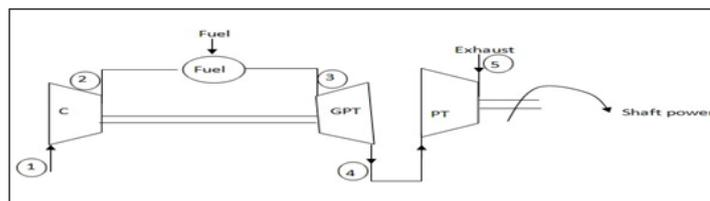
**Fig-2: Schematic Diagram of the Gas Turbine Generators**
