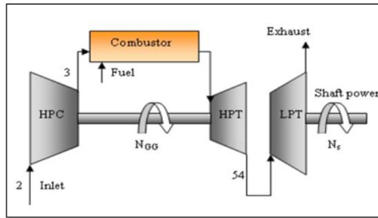
**Fig-1: Two shafted Gas Turbine with Sensor Placement**
