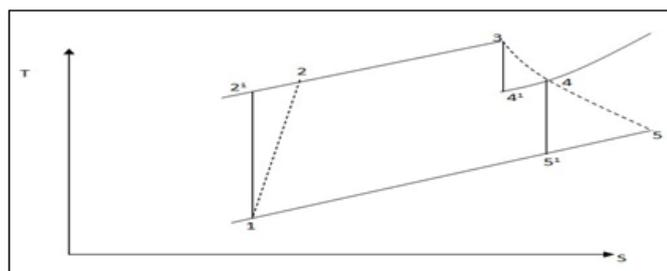
**Fig-2: T-S Diagram of the Gas Turbine Generators**
