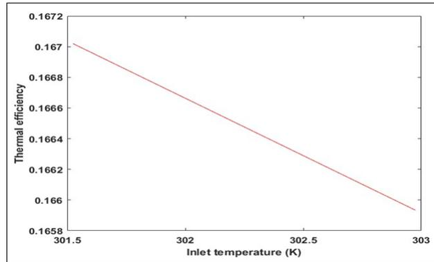
**Fig-4: Effect of Compressor Inlet Temperature on the Thermal Efficiency of the Gas Turbine Generator**
