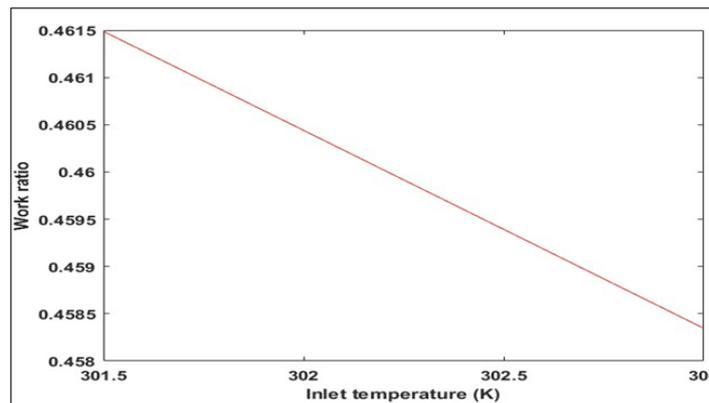
**Fig-8: Effect of Compressor Inlet Temperature on Work Ratio of the Gas Turbine Generator**
