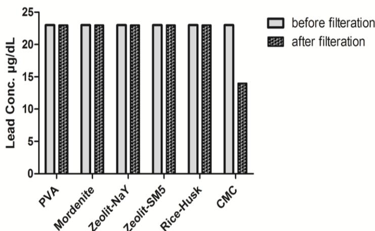
**Fig-2: Removal of Lead using different filters**
