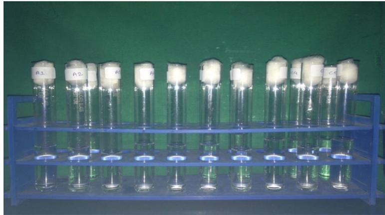
**Fig-2:** Specimen placed in a test tube containing 10 ml distilled water
