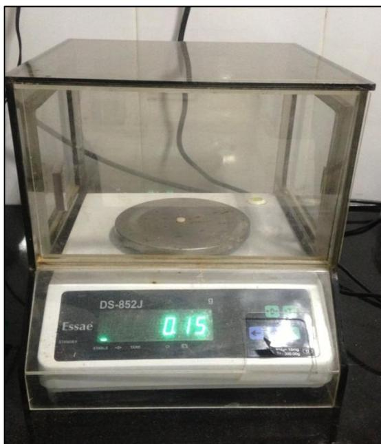
**Fig-1: Specimen placed in electrical analytical balance.**
