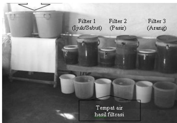
Fig- 1: Prototype equipment SPL Up flow
