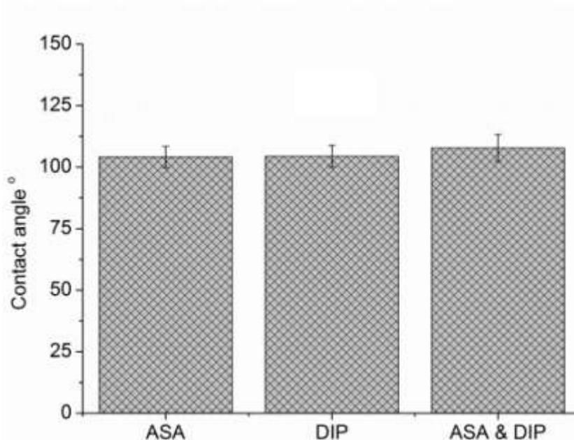
Fig 3: Static water contact angle assay for PCL/ PLA fibrous mats, with ASA, DIP and both drugs; n=5, mean ± SD.
