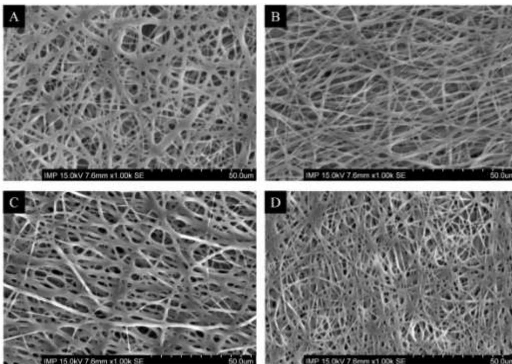
**Fig 1:** Electrospun empty PCL/ PLA fibers (A); PCL/ PLA fibers with ASA (B); PCL/ PLA fibers with DIP (C);PCL/ PLA fibers with ASA+DIP (D);magnification = 1000×, scale bars = 50μm.
