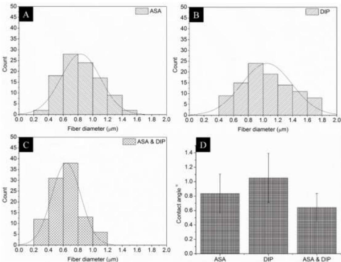
**Fig 2:** Average fiber diameter and distribution of values for PCL/ PLA fibers with ASA (A); PCL/ PLA fibers with DIP (B); PCL/ PLA fibers with ASA+DIP (C); comparative bar graphs of all specimens (D); n=100, mean ±SD.
