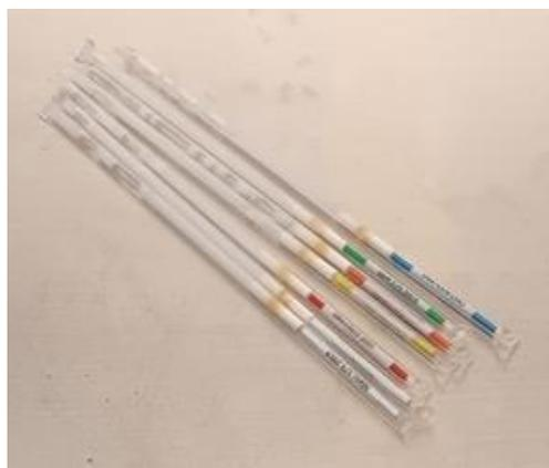
**Figure 1: High security straws (0.3ml capacity with weighted ID rod 30mm)**
