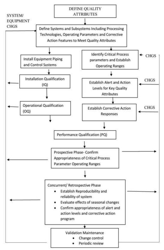
Fig-1: Water system validation life cycle
