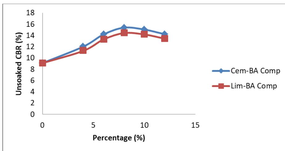
**Figure 6: Plot of CBR for unsoaked sample versus stabilized soil composites**
