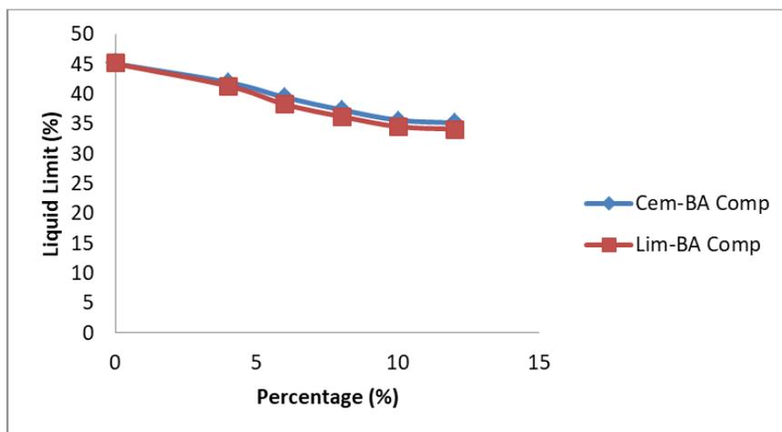
Figure 3: Liquid limit versus stabilized soil composites
