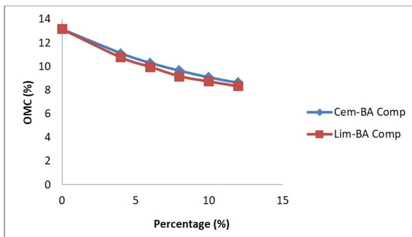
Figure 2: OMC versus stabilized soil composites
