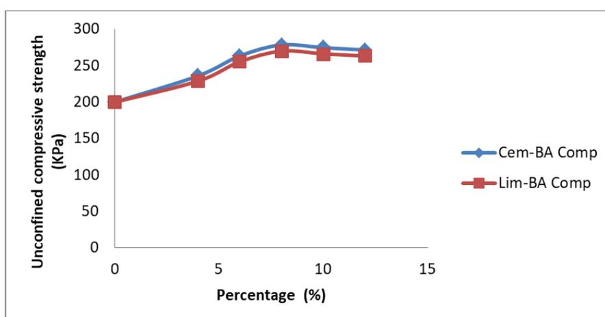
**Figure 8: Plot of unconfined compressive strength versus soil composites**
