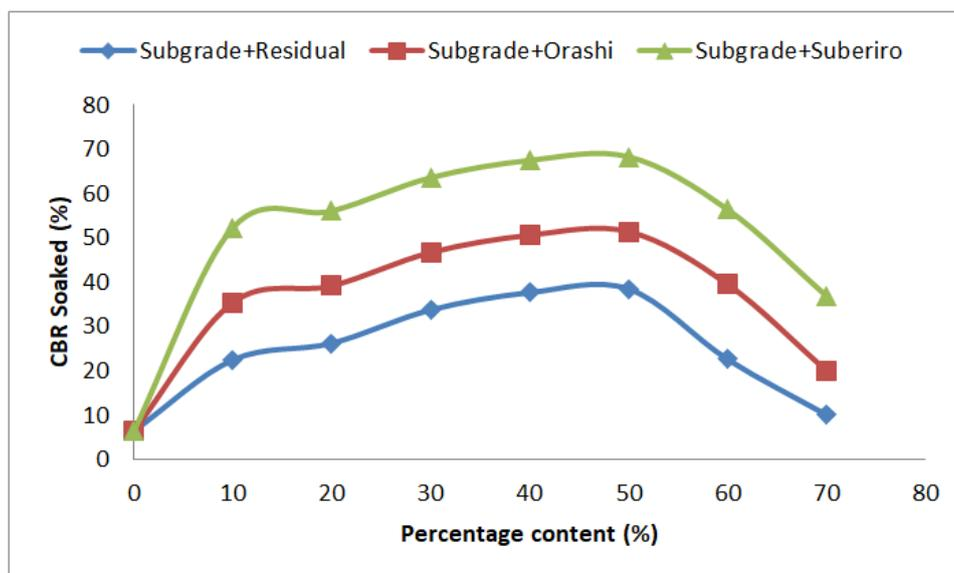
Figure 8: Comparison of CBR for soaked stabilized subgrade soil with residual soil and sand
