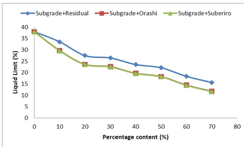
Figure 4: Comparison of liquid limit of residual soil and sand stabilized subgrade soil
