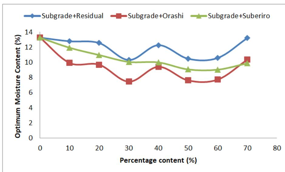
Figure 3: Comparison of OMC of residual soil and sand stabilized subgrade soil
