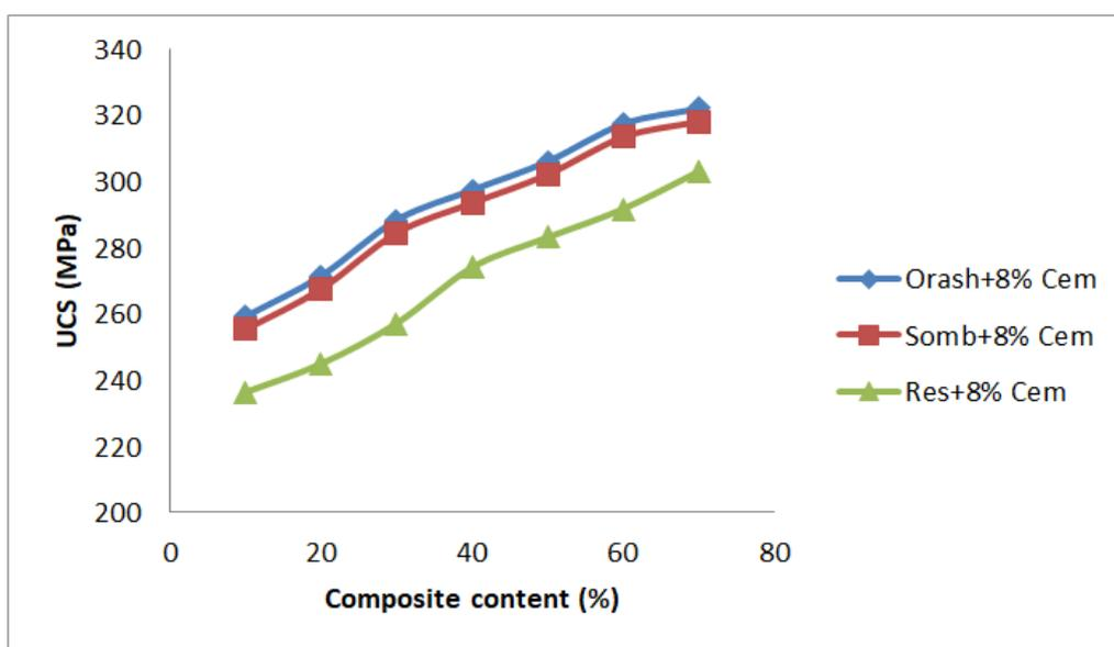
Figure 9: Comparison of UCS of stabilized subgrade soil after 7 days curing
