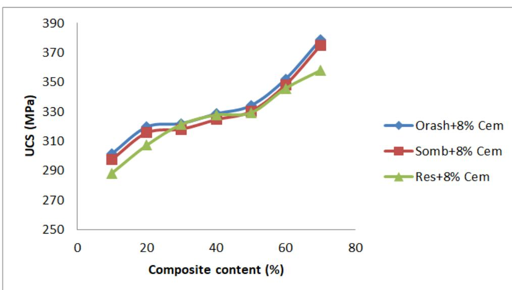
Figure 10: Comparison of UCS of stabilized subgrade soil after 28 days curing
