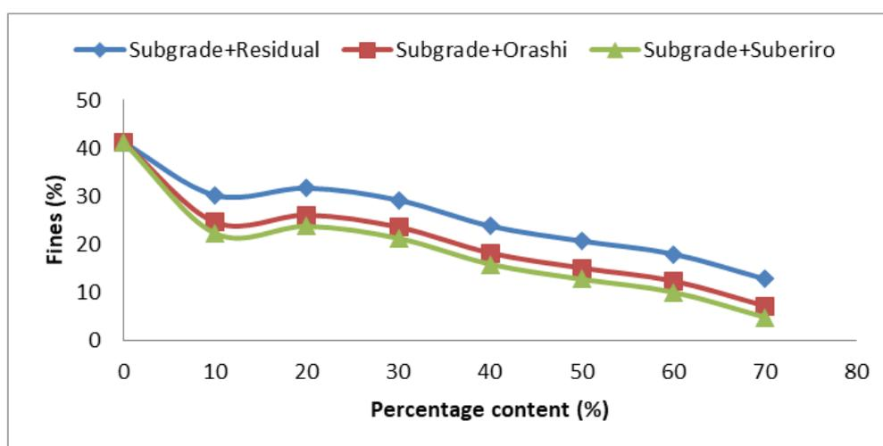
Figure 1: Comparison of fines in residual soil and sand stabilized subgrade soil
