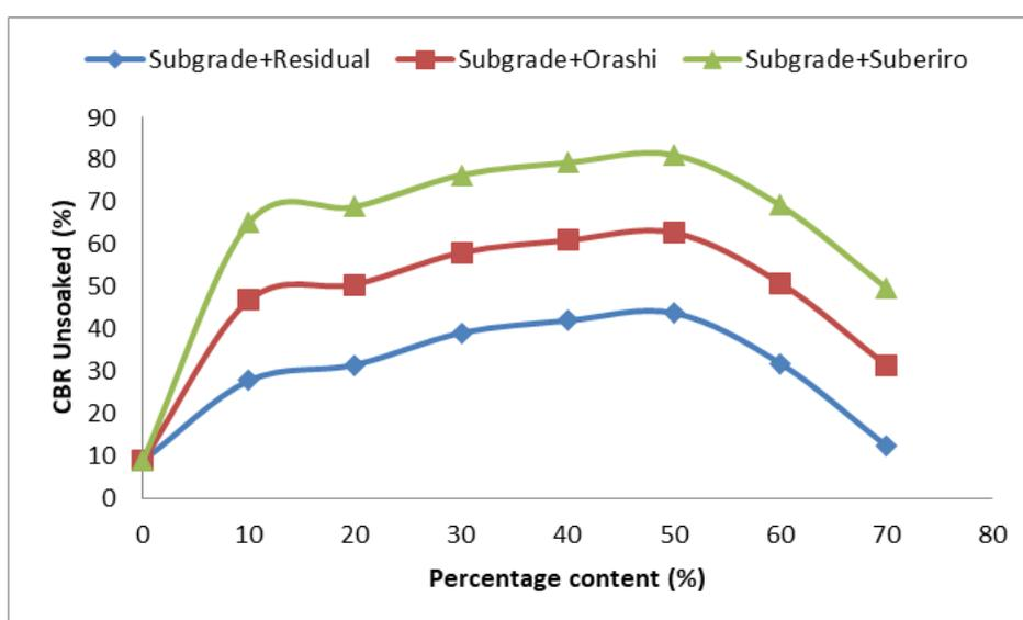
Figure 7: Comparison of CBR for unsoaked stabilized subgrade soil with residual soil and sand
