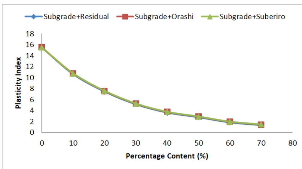
Figure 6: Comparison of plasticity index of residual soil and sand stabilized subgrade soil
