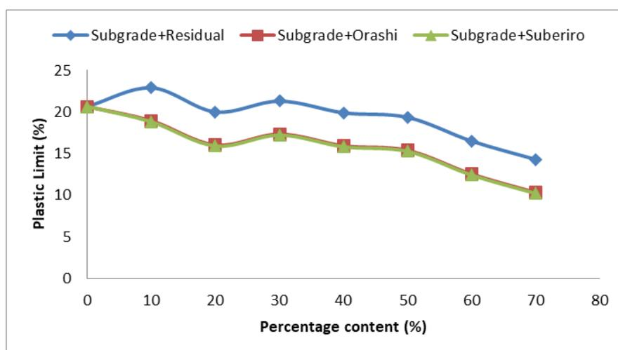
Figure 5: Comparison of plastic limit of residual soil and sand stabilized subgrade soil
