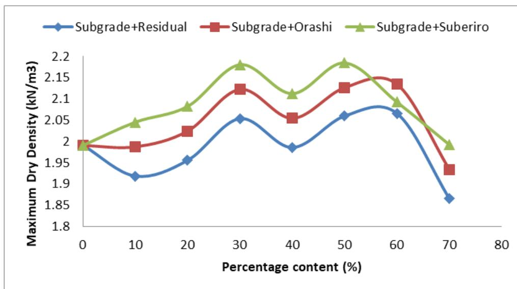
Figure 2: Comparison of MDD of residual soil and sand stabilized subgrade soil
