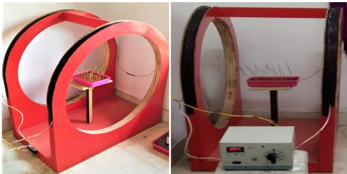
Figure 1: Helmholtz coil with base for magnetic field exposure
