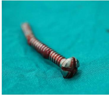
**Fig-2B:** Screw is old fashion, thought to be bended by power of magnetic field
