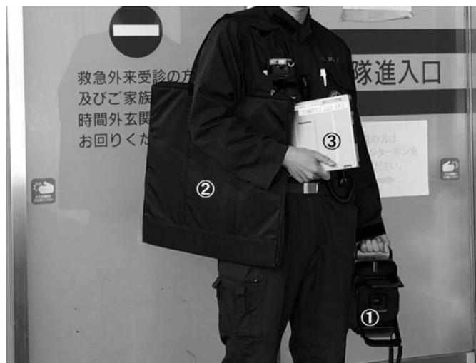
**Fig-1: CALNEO Xair<sup>®</sup> developed by FUJIFILM (Tokyo, Japan). Left: The system carried by a physician. Right: The system carried in the helicopter. (1) The X-ray radiation apparatus, (2) the special cassette, (3) a notebook-type personal computer**
