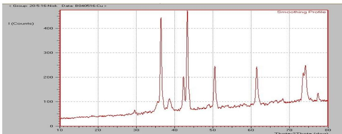
Fig-11: XRD spectrum of Copper nanoparticles (CuNP) synthesized from *Fusarium brachygibbosum*
