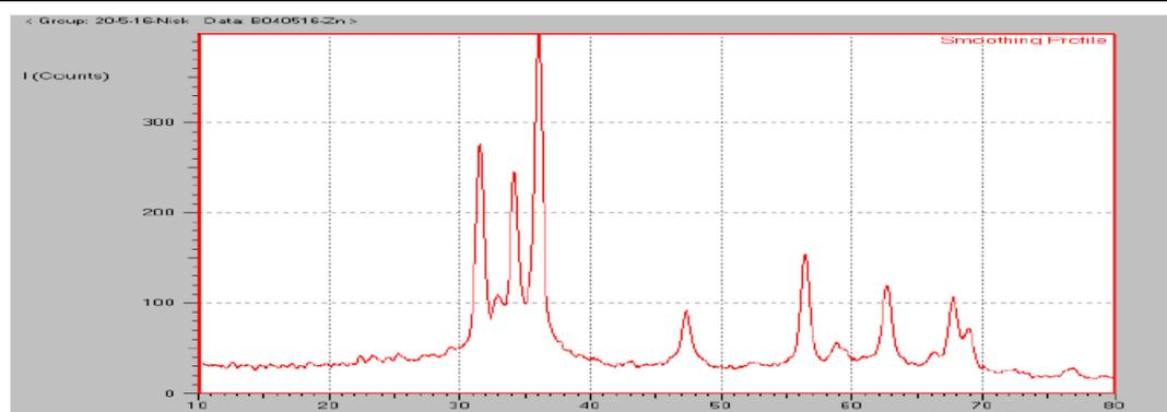
Fig-13: XRD spectrum of Manganese nanoparticles (MnNP) synthesized from *Aspergillus niger*.
