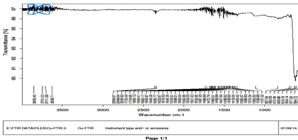
Fig-6 : FTIR spectrum of Copper nanoparticles (CuNP) synthesized from *Fusarium brachygibbosum*.
