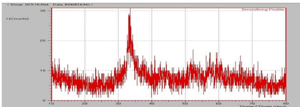
Fig-12: XRD spectrum of Zinc nanoparticles (ZnNP) synthesized from *Aspergillus niger*
