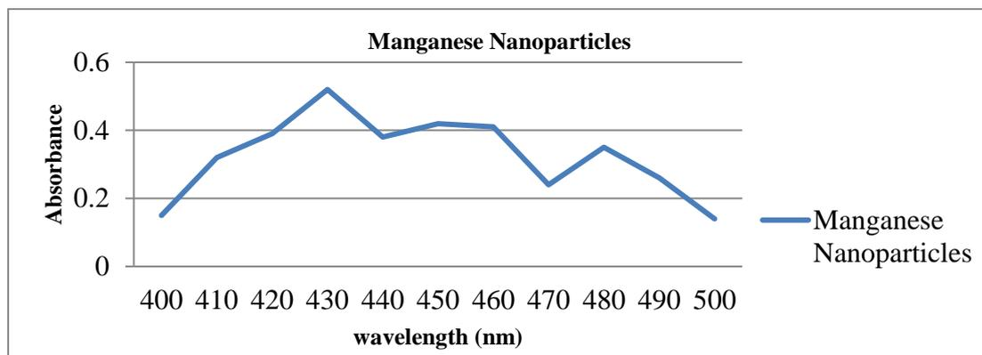
Fig-3: UV – Visible absorption spectra of Manganese nanoparticles (MnNP) synthesized from *Aspergillus niger*
