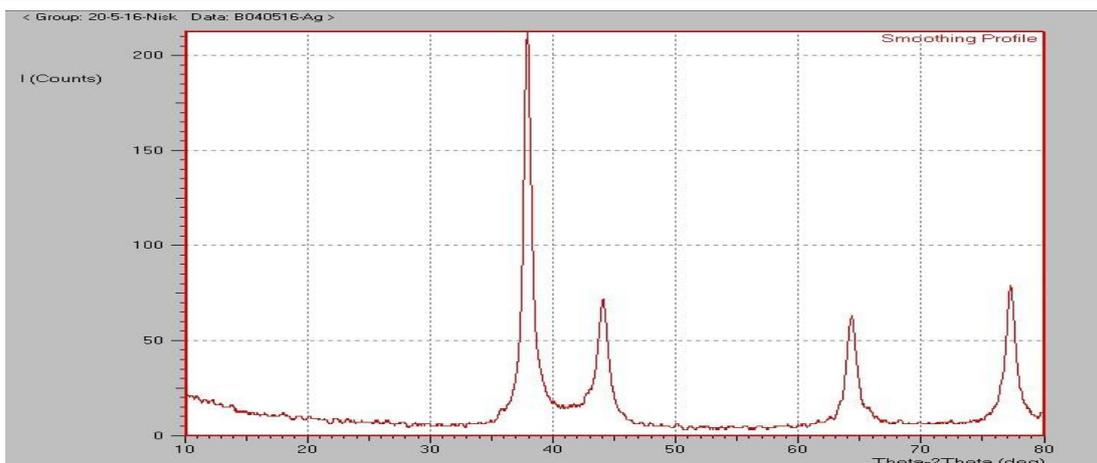
Fig-10: XRD spectrum of Silver nanoparticles (AgNP) synthesized from *Alternaria alternata*
