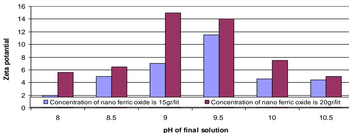
**Fig 3: Zeta potential versus final pH.**
