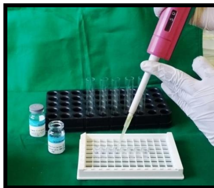
Fig-4: Addition of 50µl of standard and 50µl of streptavidin-HRP to the standard solution well.
