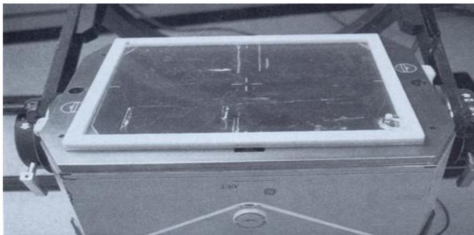
**Fig-1: An image shows a flood phantom covered the face of gamma camera where the phantom filled with <sup>99m</sup>Tc.**
