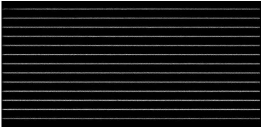
Fig-6: Gamma camera image of Parallel-line equal-space (PLES) phantom with slit equal to one mm and a distance between them equal 30 mm arranged in Y-direction
