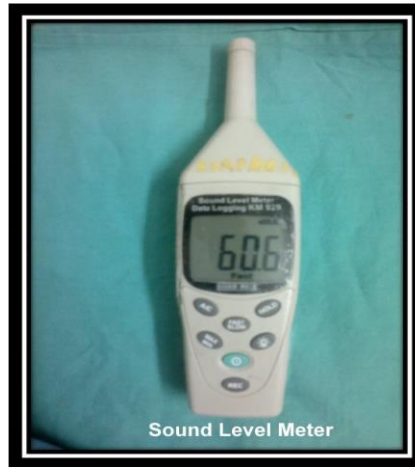
Fig-1: Sound Level Meter
