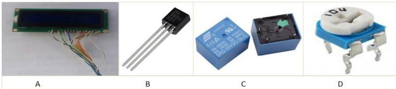
Figure 8: Liquid Crystal Display (A), Transistor (B), Relay (C), Variable Resistor (C) The Resistor R<sub>3</sub>: limits the current entering transistor Q<sub>1</sub>, MTN SIM, Light Emitting Diode, D<sub>4</sub>: indicates when the microcontroller is ready to function, Resistor, R<sub>4</sub>: limits the current entering into LED D<sub>4</sub> and Variable Resistor (RV<sub>2</sub>): for contrast and controlling the display of the liquid crystal
