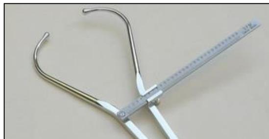
**Figure 3: Spreading caliper**
