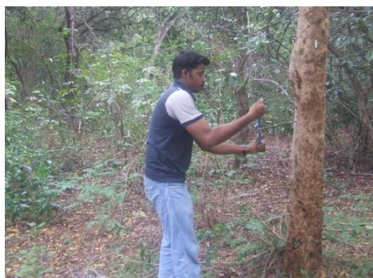
**Fig-2: Collection of wood cores with increment wood borer**
