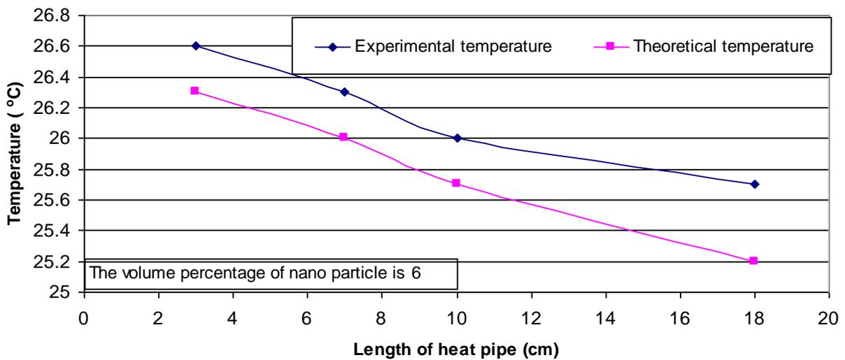
**Fig 4: Temperature profile through the pipe length at 20 W, 6% nano particles.**
