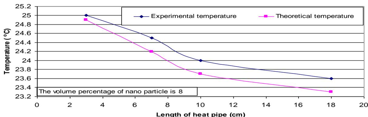
Fig 5: Temperature profile through the pipe length at 20 W, 8% nano particles.
