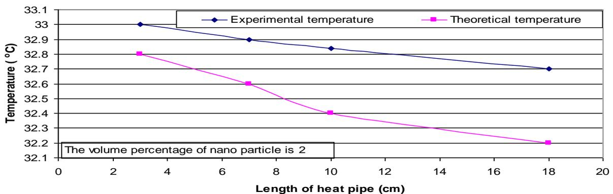
**Fig 2: Temperature profile through the pipe length at 20 W, 2% nano particles.**
