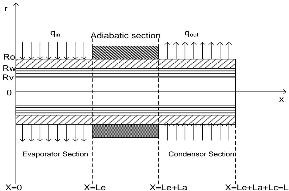
**Fig 1: The experimental heat pipe in three sections**
