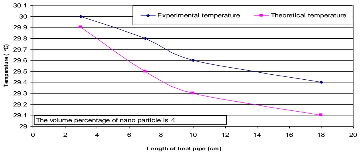
**Fig 3: Temperature profile through the pipe length at 20 W, 4% nano particles.**
