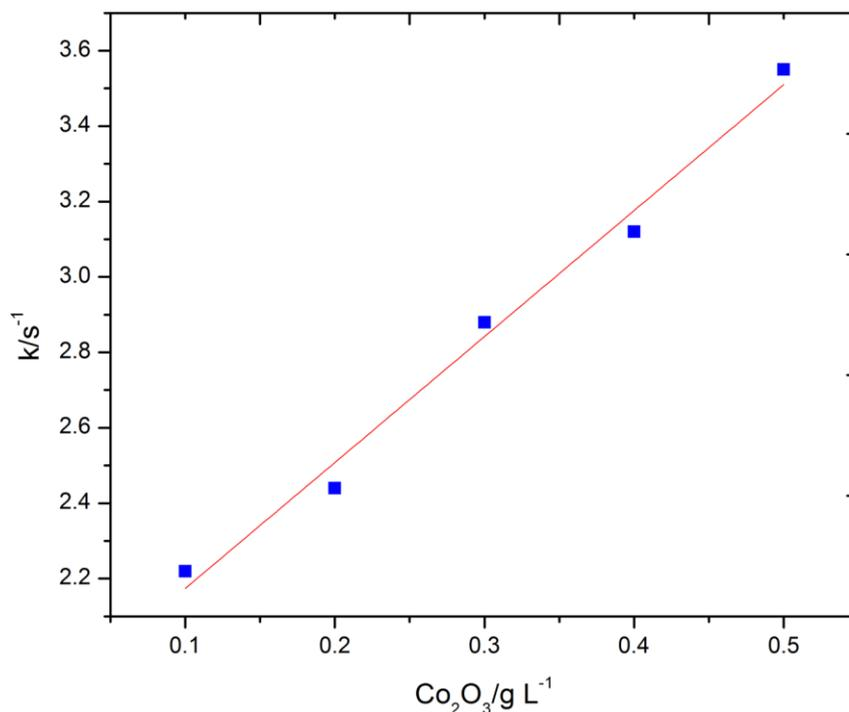
**Fig-3: Effect of  $[Co_2O_3]$  at acetic acid =  $3 \times 10^{-4} \text{ mol L}^{-1}$ , pH=7.80 and at  $t = 30^\circ\text{C}$ , in phosphate buffered medium**
