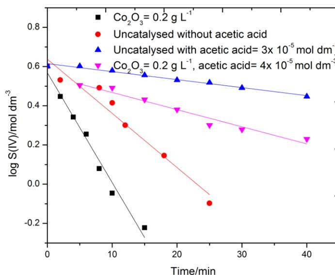
Fig-1: The disappearance of  $[\text{S(IV)}]$  with time in air - saturated suspensions at  $[\text{S(IV)}] = 2 \times 10^{-3} \text{ mol L}^{-1}$ , at  $30^\circ \text{C}$  and  $\text{pH} = 7.80$
