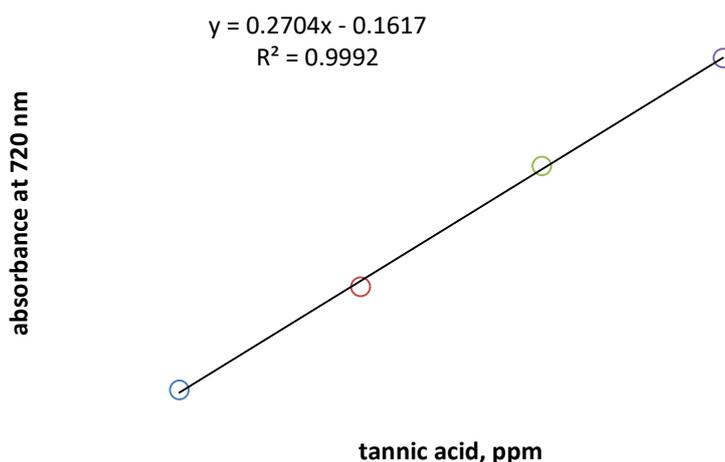
Fig-2: Calibration curve of tannic acid using Prussian blue method
