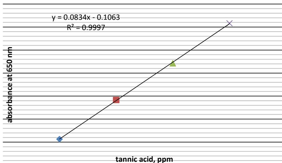
Fig-1: Calibration curve of total phenols using Folin Ciocalteu method
