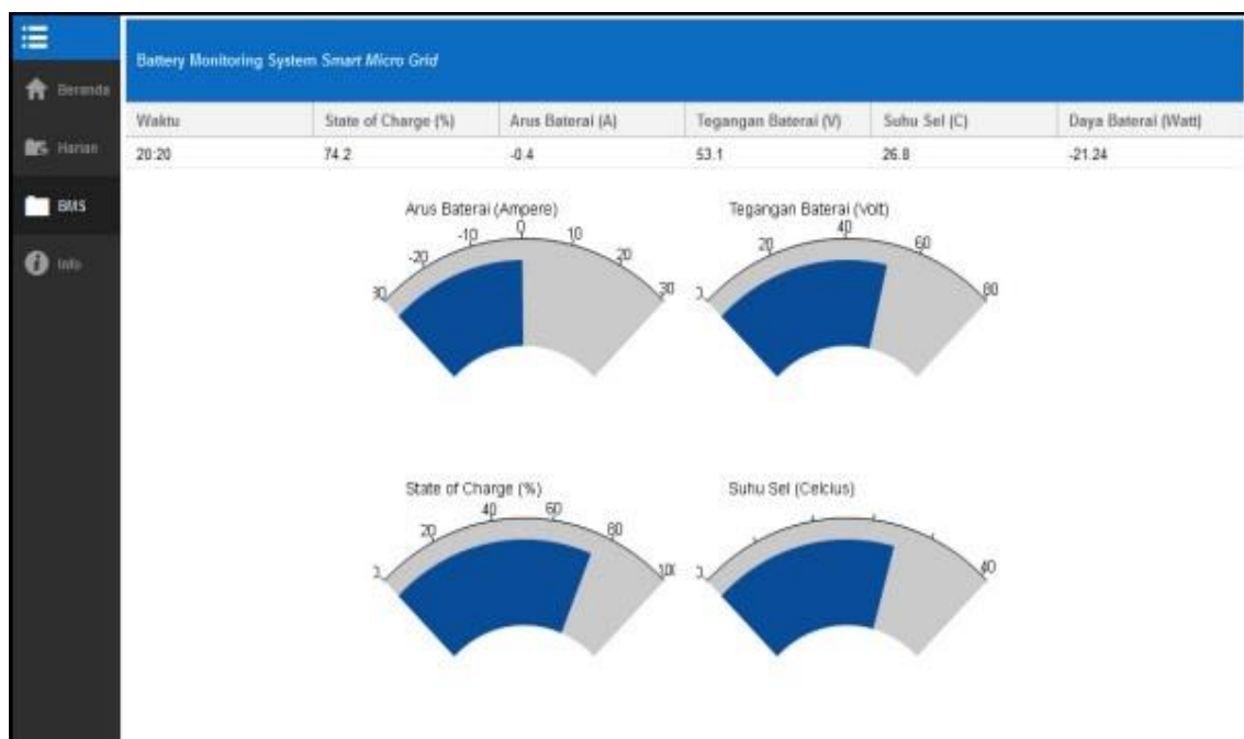
Fig. 7: GUI Monitoring of IoT Battery Pack
