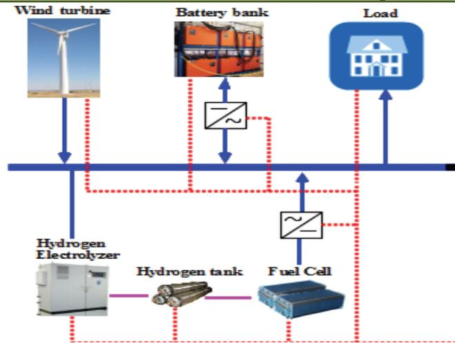
Figure 1.1: Schematic of Wind-Hydrogen-Fuel cell Hybrid System: Zachariah, *et al.*, (2013)
