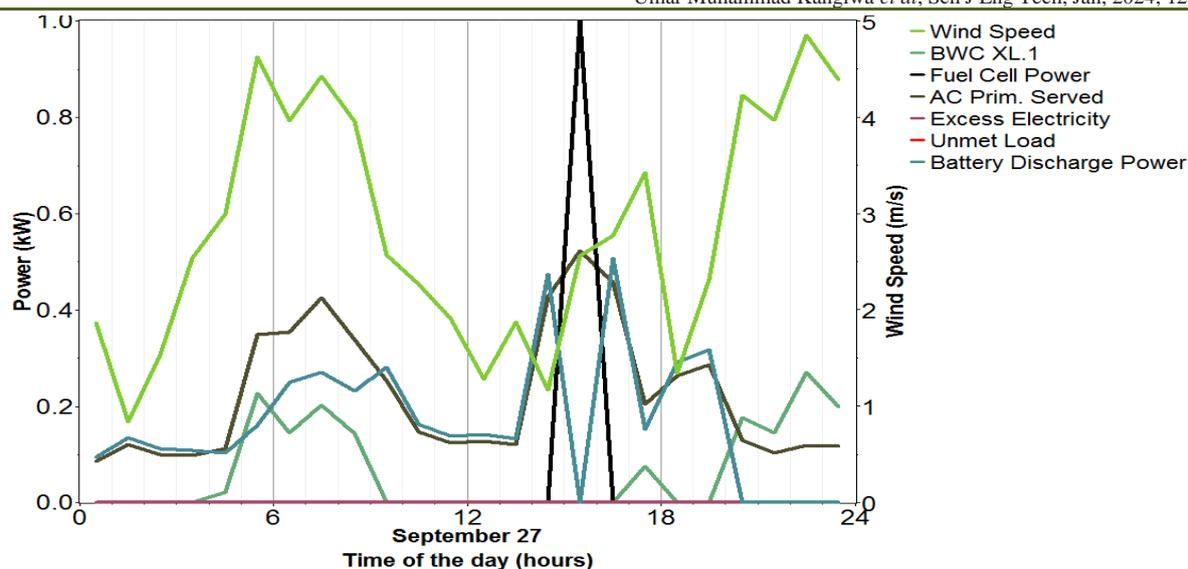
Figure 3.3: Control Strategy of Power Outputs with Respect to Wind speed
