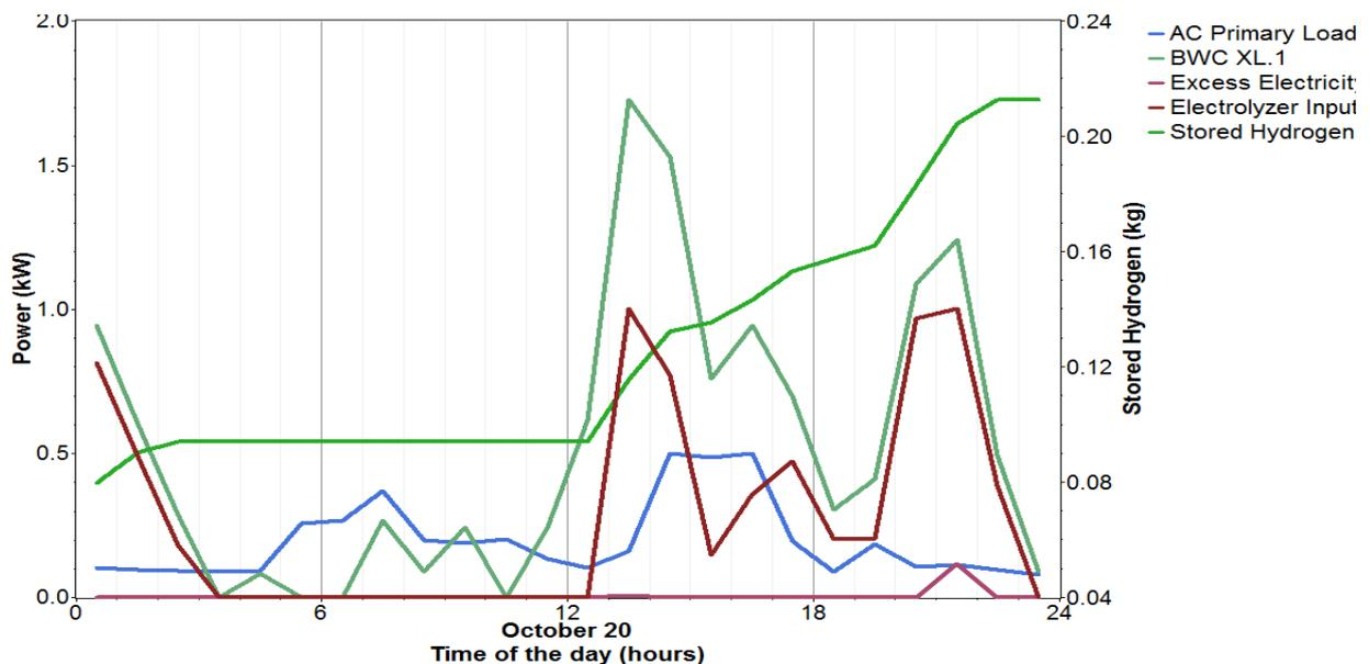
Figure 3.2: Control strategy of Power Outputs with Respect to Stored Hydrogen
